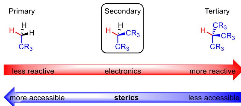
**Figure 1.9** Electronic vs steric effects of C–H bonds in C–H insertion reactions
