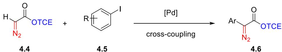
**Scheme 4.7** Synthesis of trichloroethyl aryldiazoacetates by palladium-catalyzed cross-coupling
