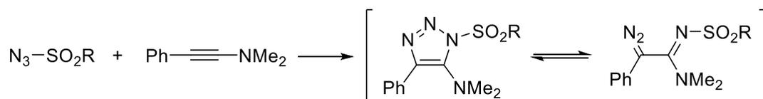
**Scheme 1.7** Triazole rearrangements/ring-chain isomerization
