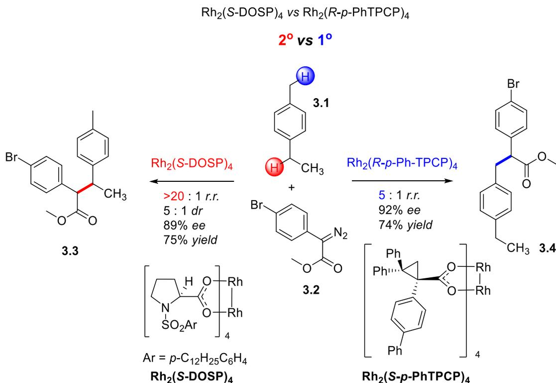
**Scheme 3.1** Site selective C–H insertion with  $\text{Rh}_2(\text{S-DOSP})_4$  and  $\text{Rh}_2(\text{R-}p\text{-PhTPCP})_4$
