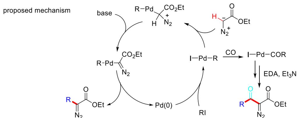
**Scheme 4.3** Wang's work on the synthesis of diazoacetates by cross-coupling
