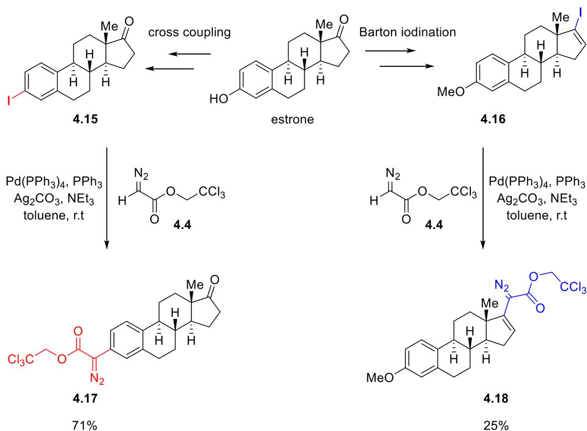
**Scheme 4.8** Application of the cross-coupling methodology to estrone derivatives
