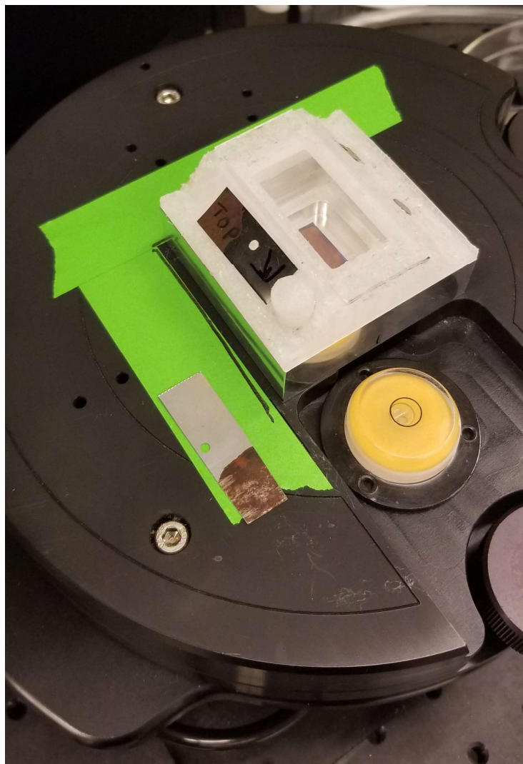
Figure 15. Photograph of the sample chamber in use on the ellipsometer.
