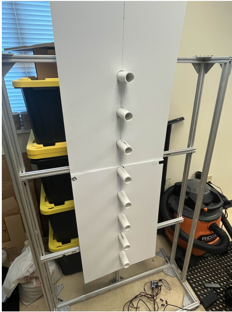
Figure 2.5: Pegboard in the 15.2 cm configuration. Aluminum T-frame behind poster-board covering allows for pegs to be slid to desired positions and held in place with screws. Poster-board cover prevents snake from getting caught behind pegs.
