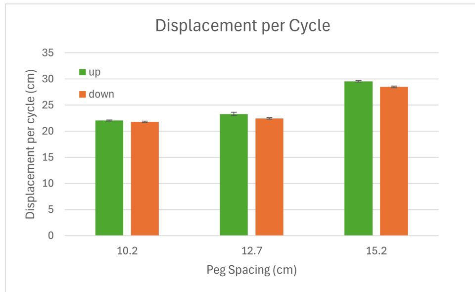
Figure 3.6: Average displacement per cycle for each peg spacing, up and down. Error bars represent one standard deviation for the ten trials used to find the average displacement per cycle for a given set of parameters.
