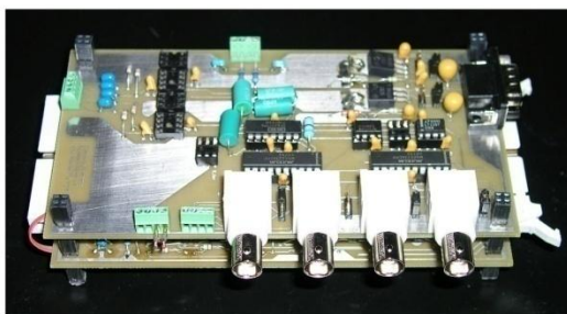
Assembled Boards, Power Board on Top
