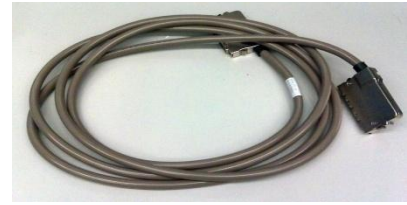
FIGURE C-2. MCS 68-pin SCSI cable.
