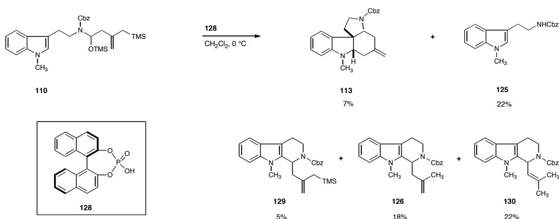
**Scheme 2.10** Cyclization of *N*-Cbz-*O*-TMS aminol **110** with protic acid.
