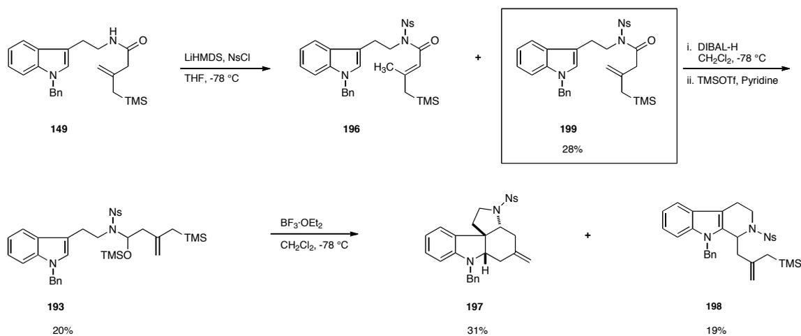
**Scheme 2.26** Synthesis and cyclization of *N*-nosyl-*O*-TMS-aminol **193**.
