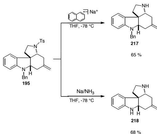
**Scheme 2.34** Protecting group removal following cascade annulation reaction.
