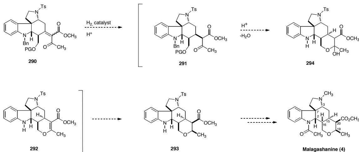
**Scheme 3.2** Proposed tandem reaction to access malagashanine from  $\alpha,\beta$ -unsaturated ketoester **290**.
