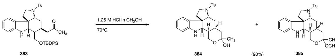
**Scheme 3.33** Hydrolysis of silyl ether **383**.
