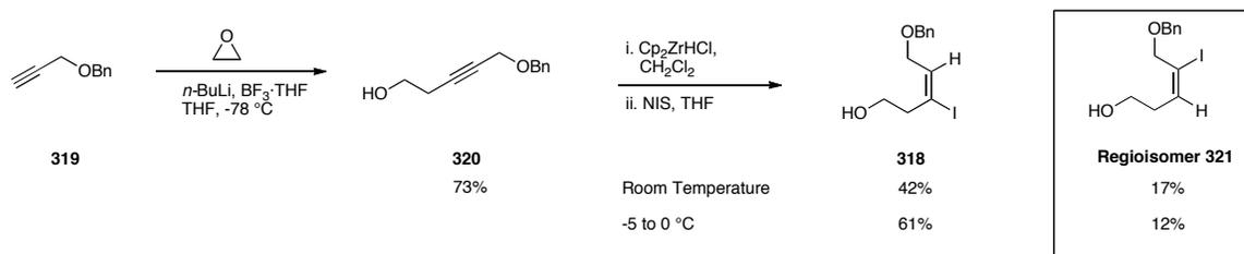
**Scheme 3.8** Second generation synthesis of iodo-alcohol **318**.
