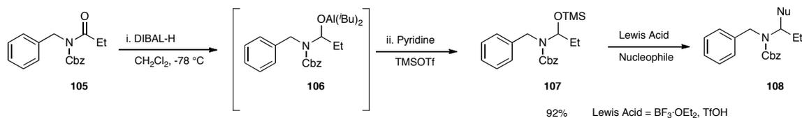
**Scheme 2.3** *N*-acyl-*O*-TMS-aminols are versatile *N*-acyliminium ion precursors.
