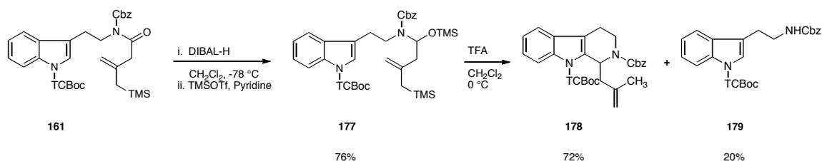
**Scheme 2.23** Cyclization of *N*-Cbz-*O*-TMS-aminol **161** with protic acid.
