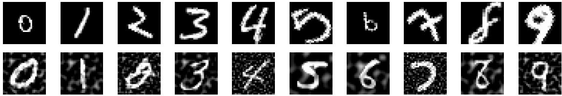
Figure 4.5: Samples from Noisy MNIST data set [2]. The data set contains \sim 56k training and \sim 7k test digit pair, X and Y . In each pair, the same digit (but its two different instances) are corrupted by scaling / rotation, X , and by background noise, Y .
