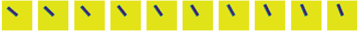
Figure 5.1: Individual frames from a physical single pendulum’s motion. The dataset and more information can be found in [35]. Each image represents a frame captured during the pendulum’s real motion. The sampling rate is 60 Hz, and each frame is 28 \times 28 pixels, with a total of 60 frames per experiment. Each experiment has different initial conditions, with a total of 1200 experiments. The pendulum is of mass of 1 kg, and a length of 0.5 m.
