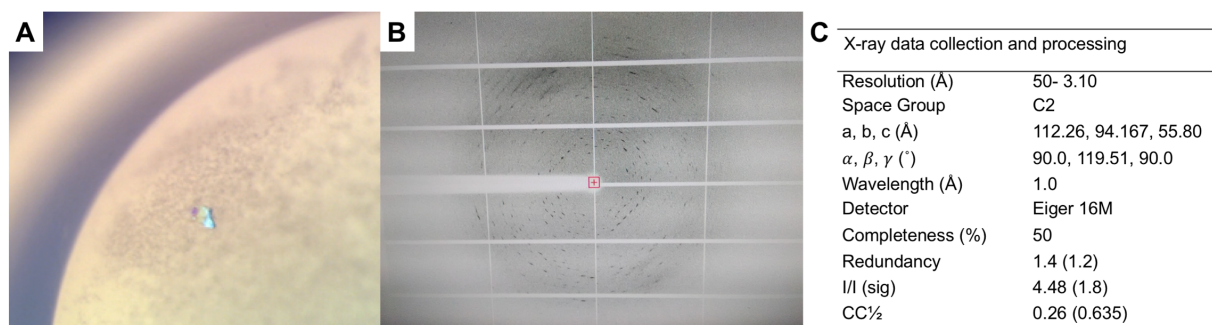
Figure. 2. Crystallization of the free TlyA-SAM complex. A. Crystal of TlyA-SAM grown in 0.095 M sodium citrate tribasic dihydrate, pH 5.6, 19% v/v 2-propanol, 19% w/v polyethylene glycol, 5% glycerol at 20°C. B. Diffraction image collected at the Southeast Regional Collaborative Access Team (SER-CAT) beamline at the Advanced Photon Source (APS) at Argonne National Laboratory. C. Initial x-ray diffraction data information and processing statistics.
