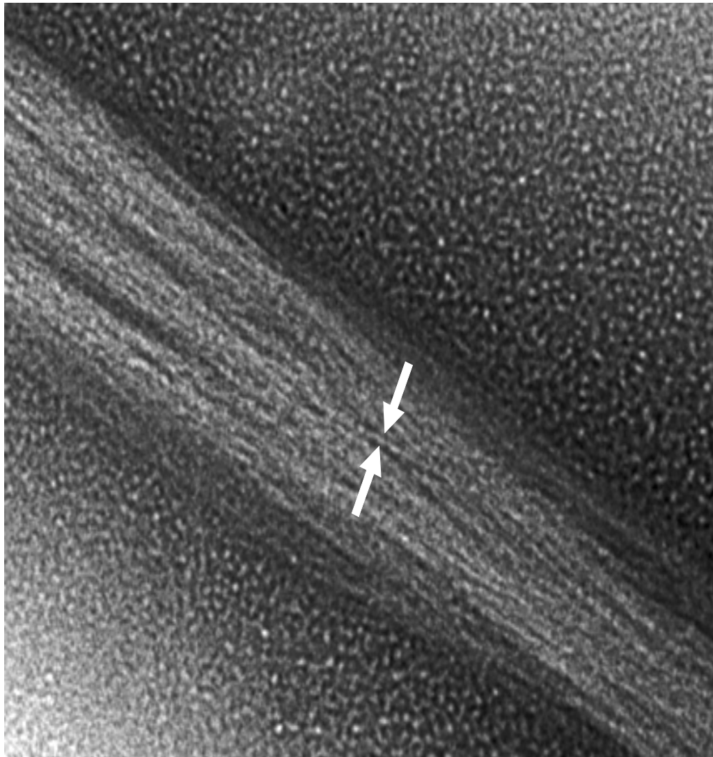
Figure 2.12. Higher magnification TEM image of large diameter bundles reveals longitudinal striations displaying diameters reminiscent of isolated small diameter fibrils.
