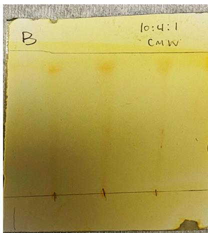
**Figure 3.8:** Glass-backed TLC Plate for Bioautography. The DCM partition was spotted three times at a concentration of 10 mg/mL. The mobile phase used was 10:4:1 CMW.
