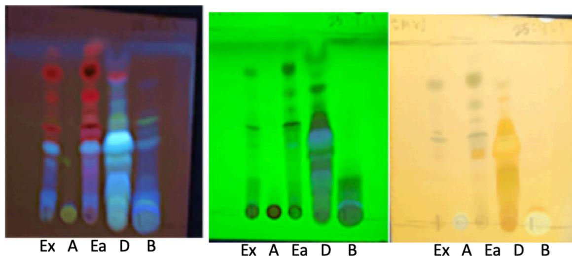
**Figure 3.3:** Example of Foil TLC spotting of samples with 10 mg/mL concentrations in the following order (left to right): Extract; Aqueous; Ethyl acetate, Dichloromethane, Butanol. The plates are visualized with UV rays at 254 nm (green) and 365 nm (blue), and after Dragendorff's spraying reagent was applied (orange). The mobile phase used was 25:4:1 CMW.
