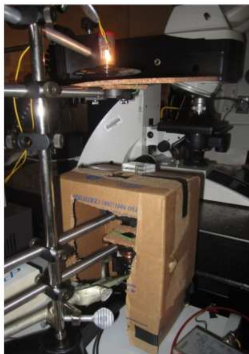
Figure 2.3: Soap film thickness measuring device used in experiments. Light from an incandescent lamp is focused on the soap film. Then the light transmitted from the soap film is incident on the IR filter that allows only light of wavelength 3 \mu\text{m} to be detected by the photodetector.
