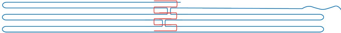
Figure 4. 6HB scaffold routing, and how seed at domain 13 and domain 14 lock the scaffold.
