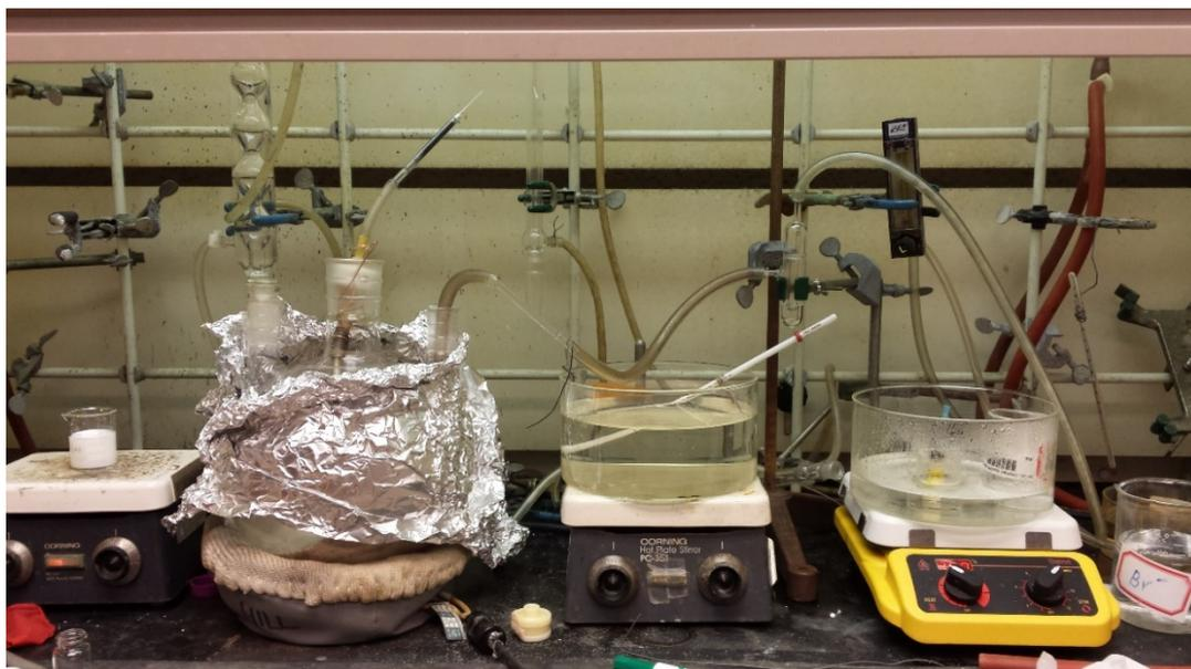
**Figure 16.** Device for assessing catalytic activity for air-based oxidation of CEES
