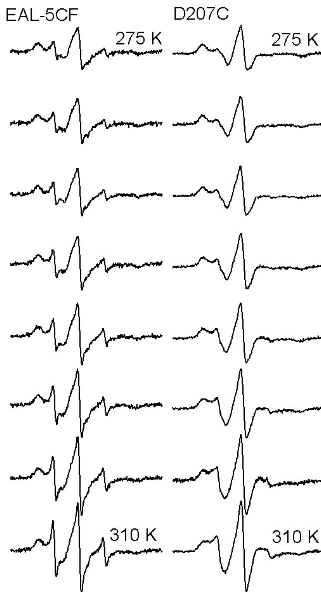
Figure 9. cw-EPR Spectra of 4MT spin labeled EAL-5CF and D207C mutants at various temperatures. (Left) 60 \mu\text{M} EAL-5CF, 120 \mu\text{M} AdoCbl, 60 \mu\text{M} 4MT. (Right) 60 \mu\text{M} D207C, 120 \mu\text{M} AdoCbl, 60 \mu\text{M} 4MT. Spectra from top to bottom are at 275 K to 310 K in 5 K steps. Spectra scaled to match integral of absorbance. Experimental parameters: Frequency, 9.452 GHz. Power, 2 mW. Modulation frequency, 100 kHz. Modulation amplitude, 2 G. Dwell time, 10.24 ms. Time constant, 2.56 ms. 49 scans.
