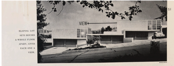
Figure 17: View of Avenel Homes from the street. Gregory Ain, Architect. Pictured with the caption: “Sloping Lot Sets Houses a Whole Floor Apart, Gives Each One a View,” from “A Step-back Plan on a Hillside Site Gives Privacy to Ten Los Angeles Families,” House and Garden , February 1951, 51.
