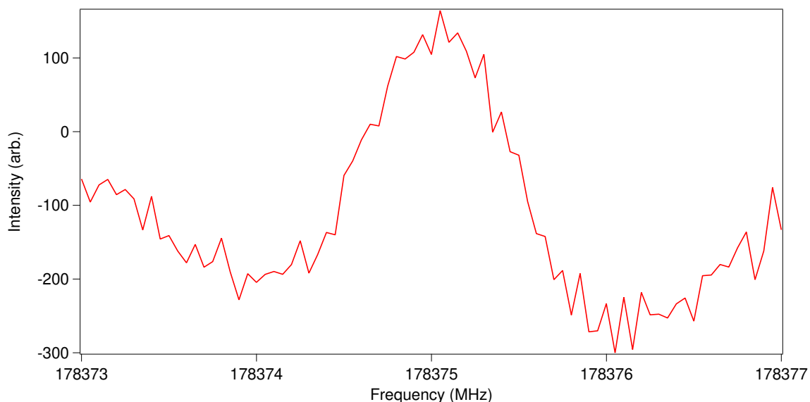
Figure 4.12: The 2 \leftarrow 1 formylium transition recorded at 178375.056 MHz using lock-in detection with 10 averages. The sensitivity was set to 2 mv, the time constant was 10 ms, and the frequency step size was 0.05 MHz. The increase in step size was done in order to speed up data collection.
