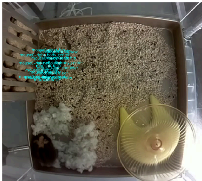
Figure 10: Example frame with incorrect mouse body part points. Only the body parts of mouse 0 are identified properly. Not a single body part of mouse 1 is identified in the bottom left corner of the enclosure.
