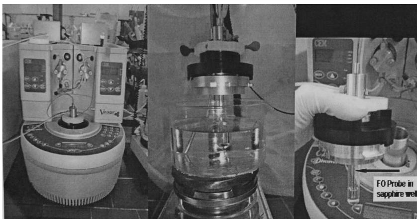
**Figure 3.** The temperature measurement using internal fiber optic probe
