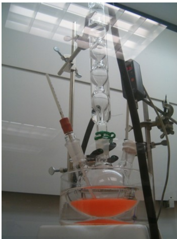
Figure 2.1: Photograph of flask and condenser used to polymerize methylmethacrylate into coiled, spherical polymer chains. The sample is bright pink because it is saturated with fluorescent dyes, guaranteeing homogeneously dyed, bright fluorescent spherical particles.
