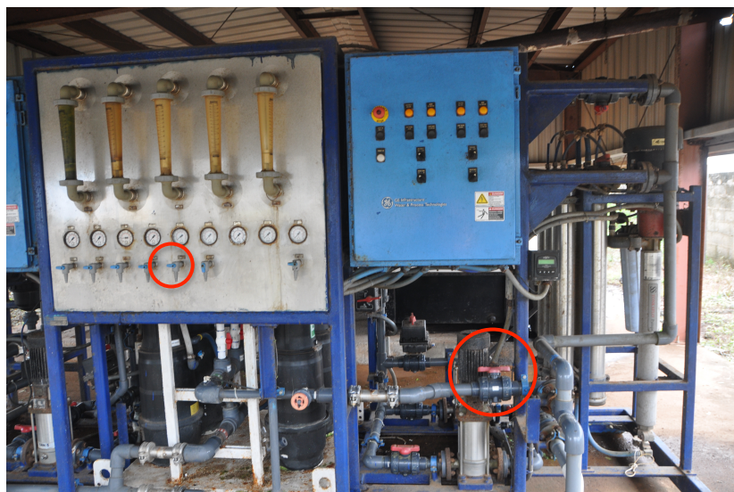
Figure 4: Raw water and filtered water sample sites for hospitals with membrane filters.
