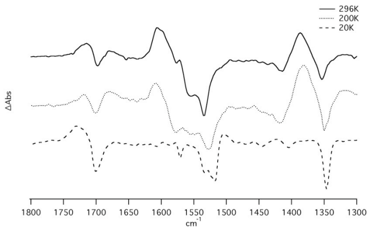
Figure 13. Light versus dark spectrum of NBA and ammonium acetate solution in \text{D}_2\text{O} at 200K
