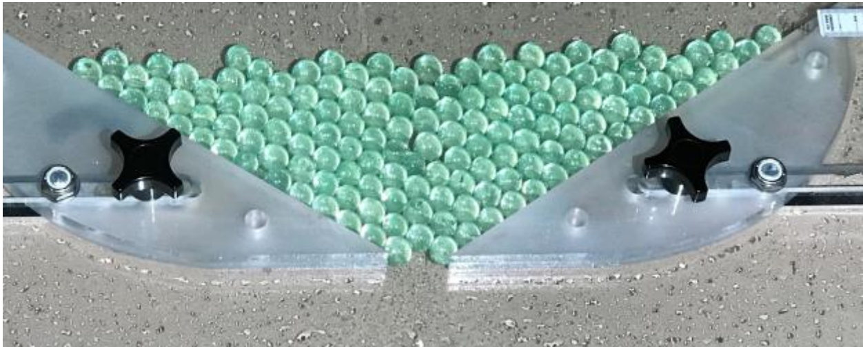
Figure 10, a clogged system at 15° inclination angle, with an opening w/d = 2.23
