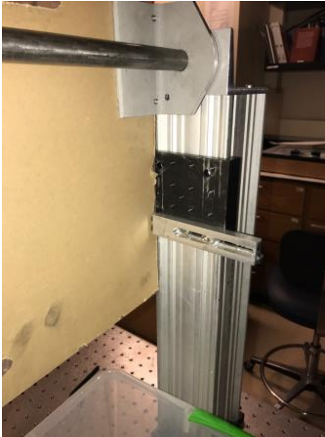
Figure 8, the stop mechanism. Here it was set at 90°. The black plastic plate can be move up and down and the metal bar can be screwed at different position in order to get the right angle.
