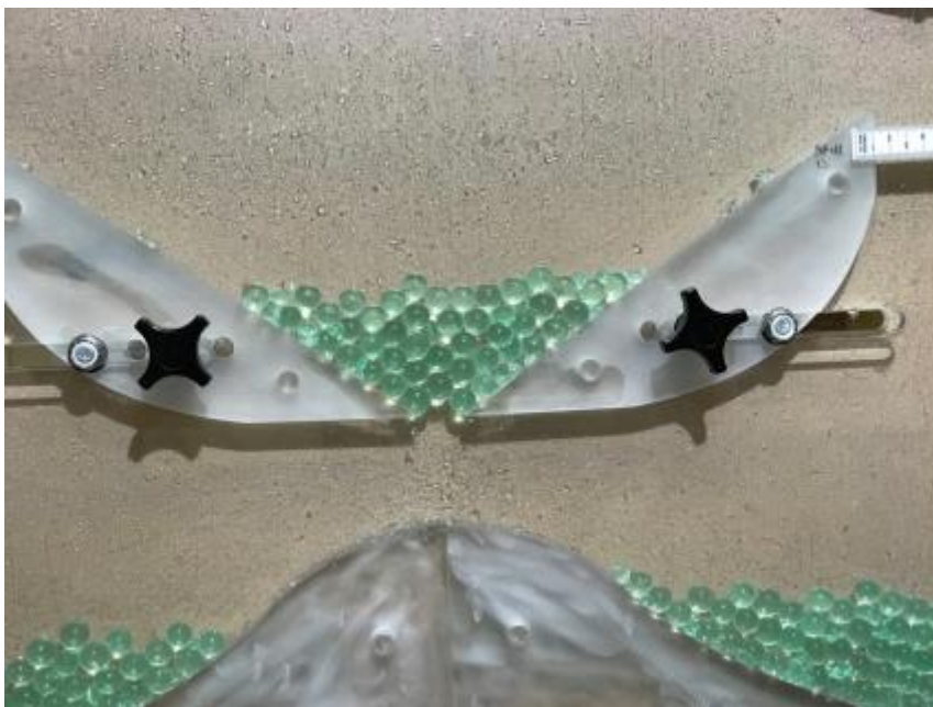
Figure 11, a clogged system at 90° inclination angle, with an opening w/d = 1.59
