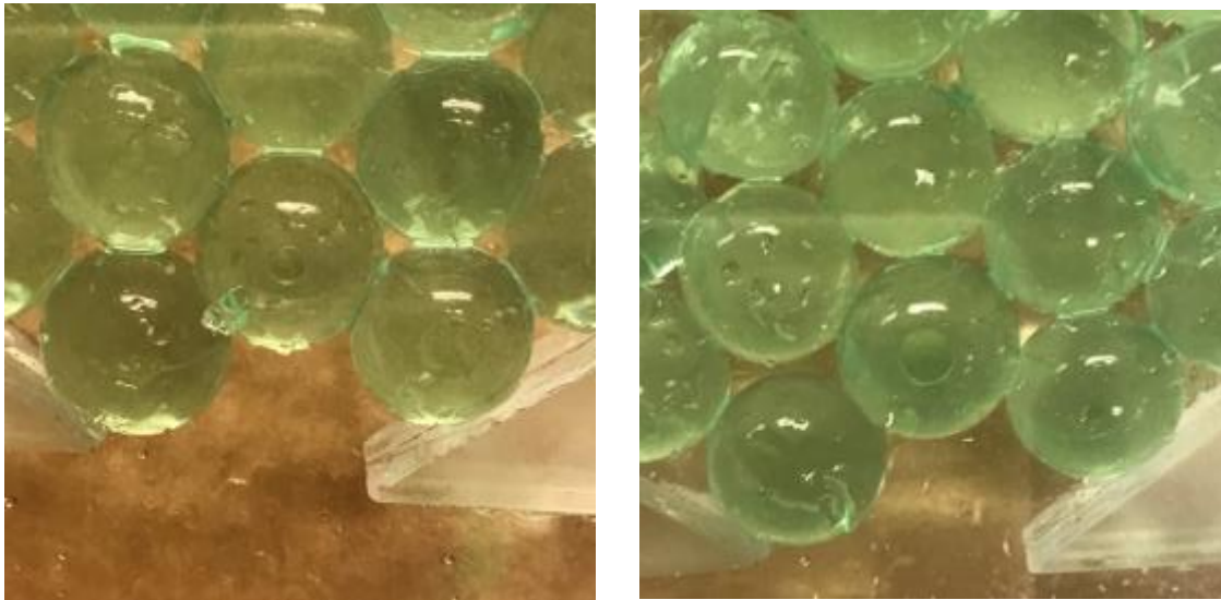
Figure 12, the two close-ups at the arches at different inclination angles. The figure on the left is the system at 90^\circ and the figure on the right is the system at 15^\circ . It is clear to see that the particles on the left figure, especially the one at the bottom right, deformed much severely than the one on the right figure at the same position.
