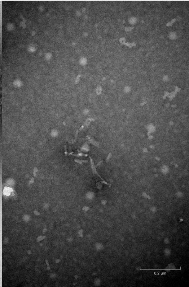
Figure 8. A) TEM image taken at 3 hours of what appears to be fibrous structures growing out of a cluster of peptide aggregates. B) TEM image taken at 24 hours shows faint outline of fibrous structures.
