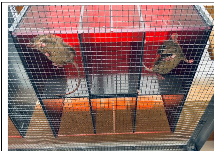
Apparatus 2. Diagonal bottom-up view of the von Frey chambers on a mesh wire table top. Mice were placed in individual chambers with opaque acrylic barriers. This configuration limited possible interferences during the test. Mice were allowed to acclimate and calm before the test started.
