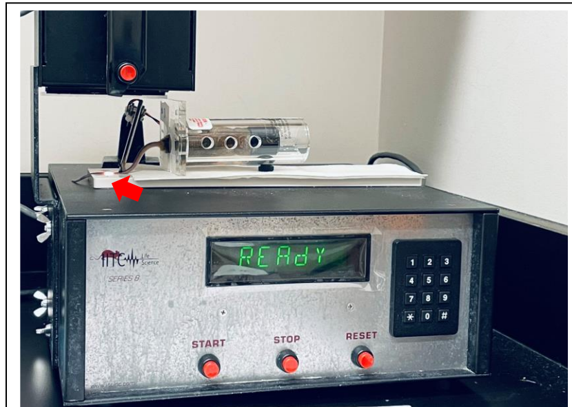
Apparatus 3. The Tail-Flick Analgesia Meter with a mouse in the semi-restraining tube, ready to be tested. The red arrow points at the focus of light that shines at 1.5 inches from the tip of the tail. After each trial, the withdrawal latency and temperature are shown on the screen in green.
