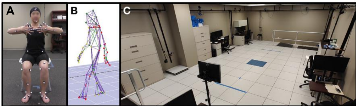
Figure 1. Clinical Motion Capture Facility. (A) Markers placed on anatomical landmarks enable measurement of their position throughout the gait cycle. (B) After data collection, software identifies and triangulates marker positions. (C) The motion analysis facility at Emory University.
