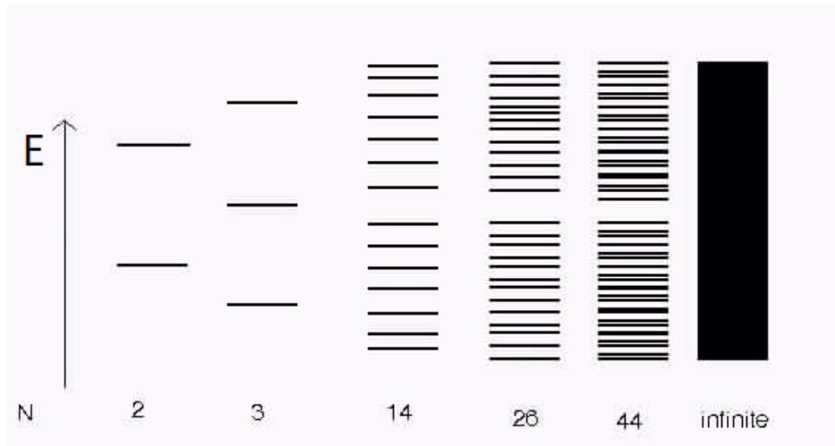
Figure 1.2: When N atoms are brought together, the distinct electronic orbitals split into N sublevels. When N is large, the sublevels can be approximated as a continuous ‘band’ of allowable energy levels
