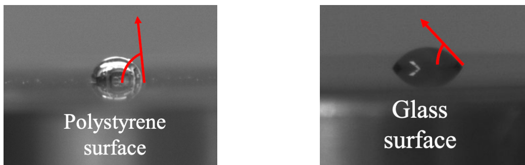
Figure 3.7: Observed contact angles on polystyrene and glass surfaces. Polystyrene (pictured on the left) is hydrophobic, observed \chi \approx 90^\circ . Glass (pictured on the right) is known to be hydrophilic, observed \chi \approx 30^\circ .
