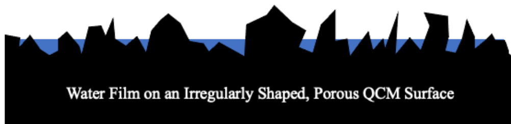
Figure 3.10: Water film formation on a porous surface. The porous material has cavities and channels where water and air can invade. A porous surface has a higher wettability than nonporous surfaces.
