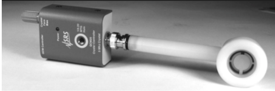
Figure 3.3: A quartz crystal microbalance [25]. The circular shaped crystal vibrates at a resonate frequency. According to the Sauerbrey Equation, as mass accumulates on its surface, the rate of oscillation slows.
