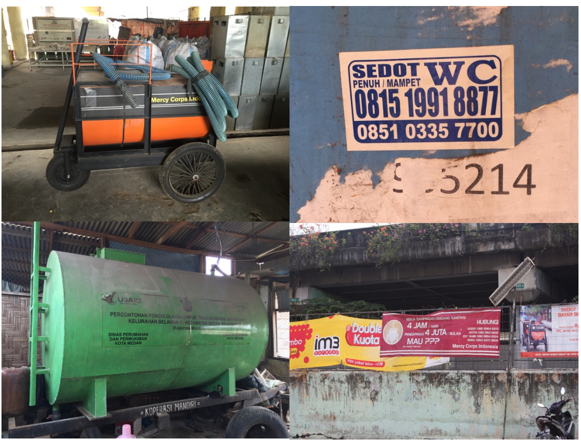
As seen in the top and bottom left, desludging services were present in many of the study sites, although the large desludging pump truck likely lacks the ability to reach households in dense areas and housing over water. The top and bottom right figures show advertisements for desludging services in Jakarta, highlighting the potential for household awareness of the need for and service options for desludging.
