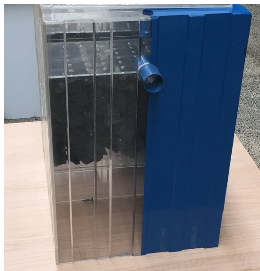
Figure 10. Type 1 Model – 3-filter septic tank
