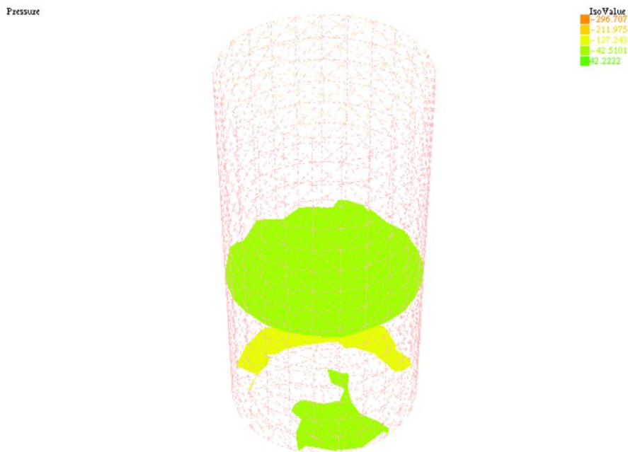
Figure 4.1: This is an example of the fine mesh that is going to be used in this experiment, the dotted lines describes the boundary of those tetrahedrons and they are where the solutions are derived.
