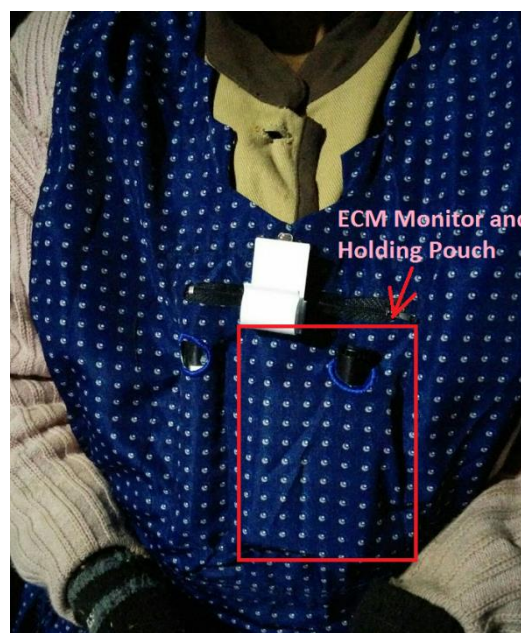
Figure 3. Apron developed by a previous Hopkins research team in Peru holding an ECM Monitor
