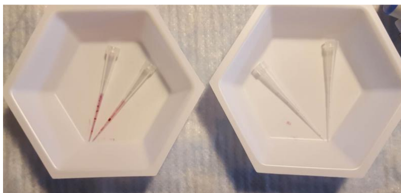
Figure 3.3 Pipette tips after transfer of DHFR-15 nm AuNP without Tween 20 (left) and with Tween 20 (right). The pink stain on the pipette tips is indicative of the conjugates sticking to the lo-bind pipette tips that were used throughout the experiments.
