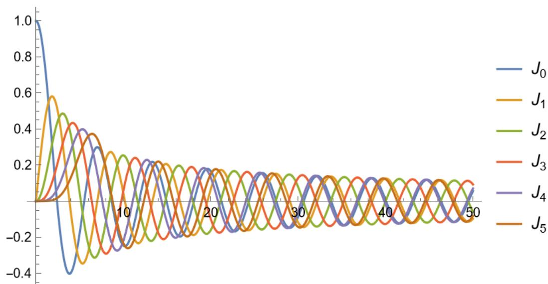
Figure 53. Bessel functions of the first kind  $J_n$  for  $n = 0, 1, 2, 3, 4, 5$ .
