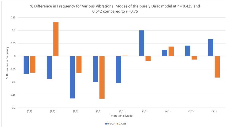
**Figure 14.** % Difference of Various Vibrational Modes of the purely Dirac model at 0.425r and 0.642r compared to 0.75r
