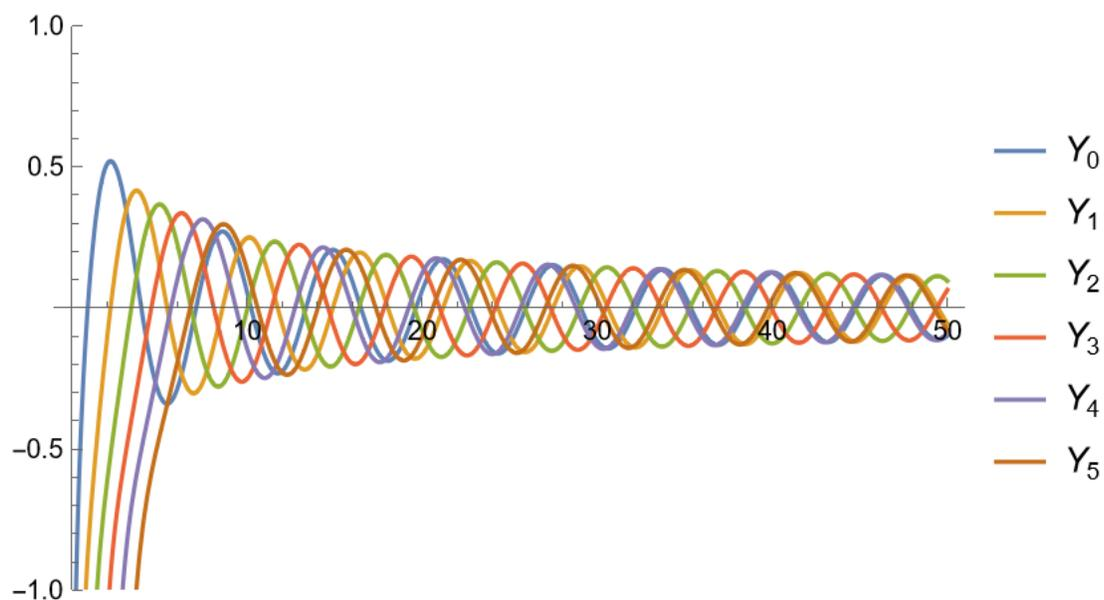
Figure 54. Bessel functions of the first kind  $Y_n$  for  $n = 0, 1, 2, 3, 4, 5$ . Note how there is always a singularity at  $x = 0$ .
