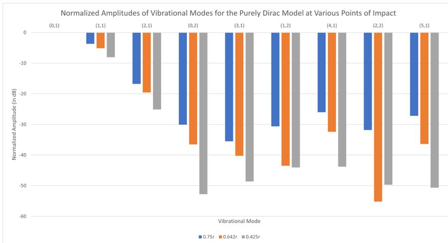
**Figure 15.** Normalized Amplitudes of Various Vibrational Modes for the purely Dirac models at Various Points of Impact
