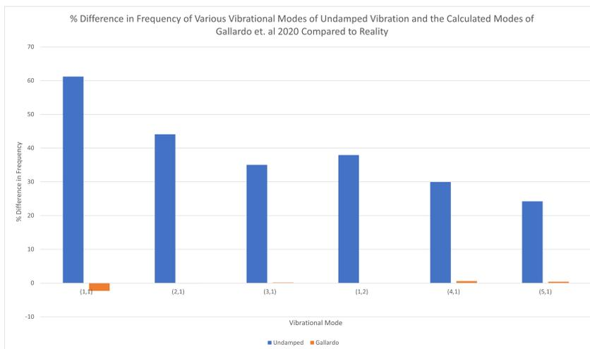
**Figure 17.** Percent Difference in Frequencies of Various Vibrational Modes of Undamped Vibration and the Calculated Modes of Gallardo et. al 2020 Compared to Reality
