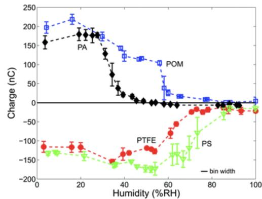
Figure 1.7: Impact of humidity levels on tribo-electric charging of polymer spheres [3]
