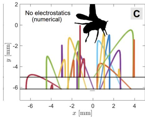
Figure 1.4: Trajectory of Nematode to fruit flies without electrostatics [2].
