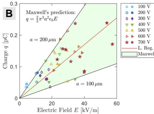
Figure 1.6: Inferred charge on a jumping nematode predicted by trajectory fitting as a function of electric field. The shaded region represents Maxwell’s prediction as stated by Equation 1.2
