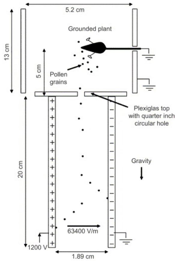
Figure 1.1: Pollen Charge Measurement Experimental Set-Up [1]
