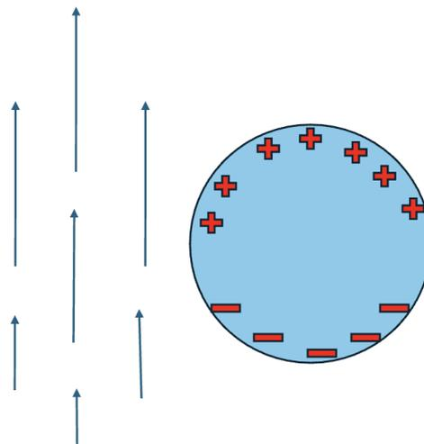
Figure 4.2: Induced polarization force on the sand grain due to an electric field gradient
