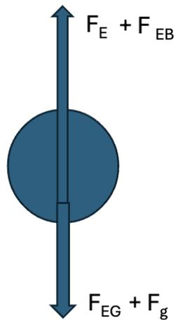
Figure 2.3: Force diagram for the sand grain
