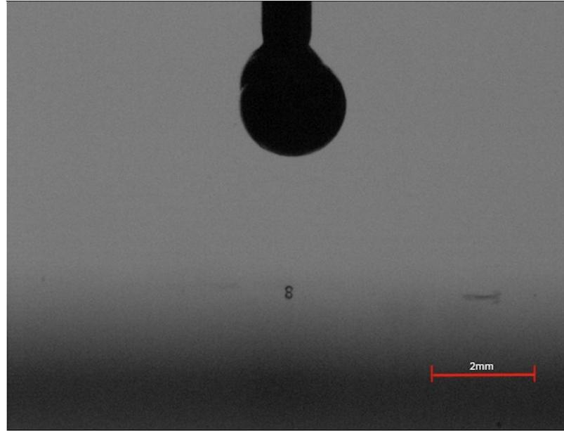
Figure 3.2: Grain under the copper sphere shown using the high speed camera
