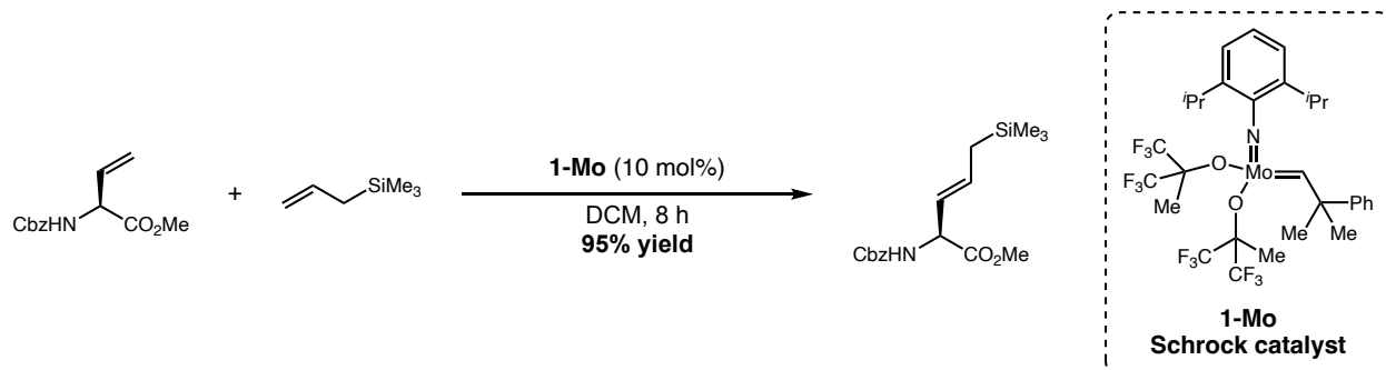
Scheme 5.23 Schrock catalysts have been employed to effectuate CM of protected vinylglycine.
