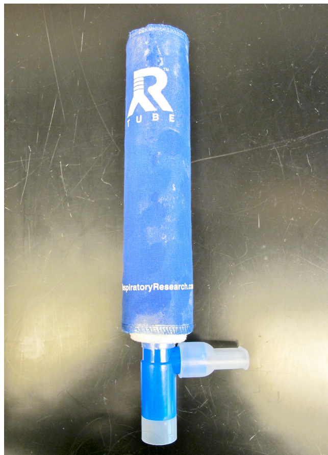
Figure 1. RTube (Respiratory Research, Charlottesville, Virginia, USA). The RTube is a portable EBC collecting system that consists of a disposable polypropylene condensation chamber with an exhalation valve, which also serves as a syringe-style plunger to pull fluid off the condenser walls. Cooling is achieved by placing an aluminium cooling sleeve over the disposable polypropylene tube. 30
