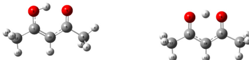
(a) Acetylacetone (AA); Global minimum(GM) (left) and the Transition State (TS) (right)
