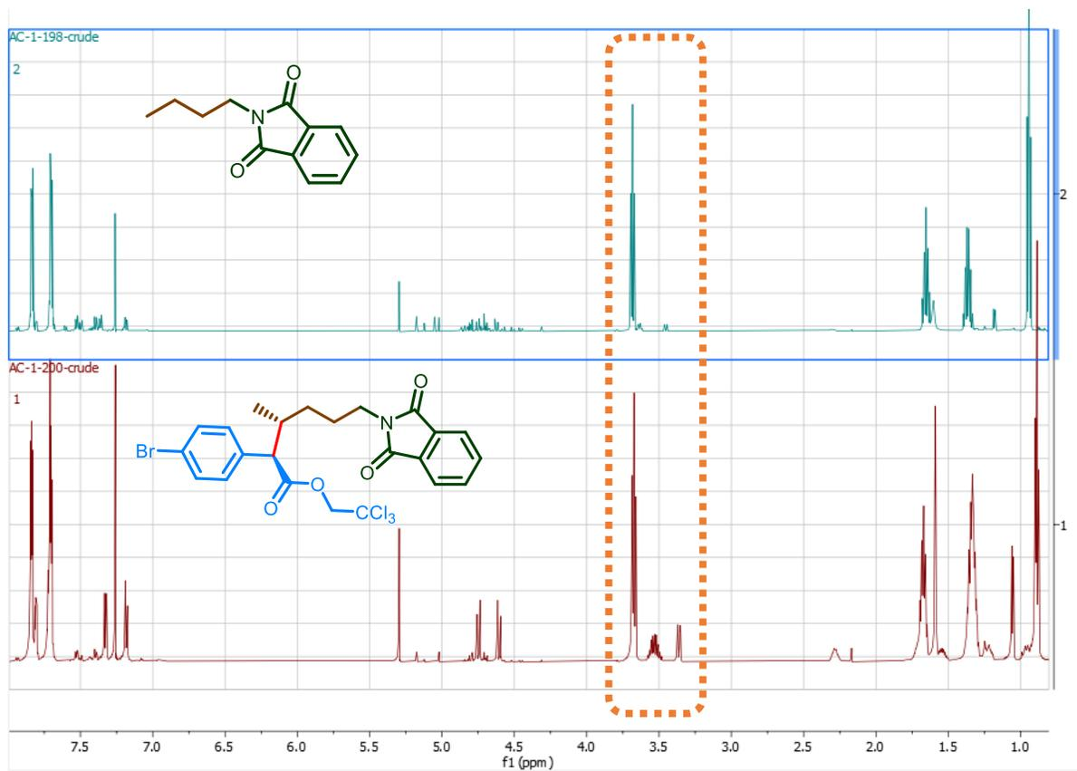
**Figure 2.11 Comparison between Crude NMRs for the Reaction with Pentylamine and Butylamine Derivative**
