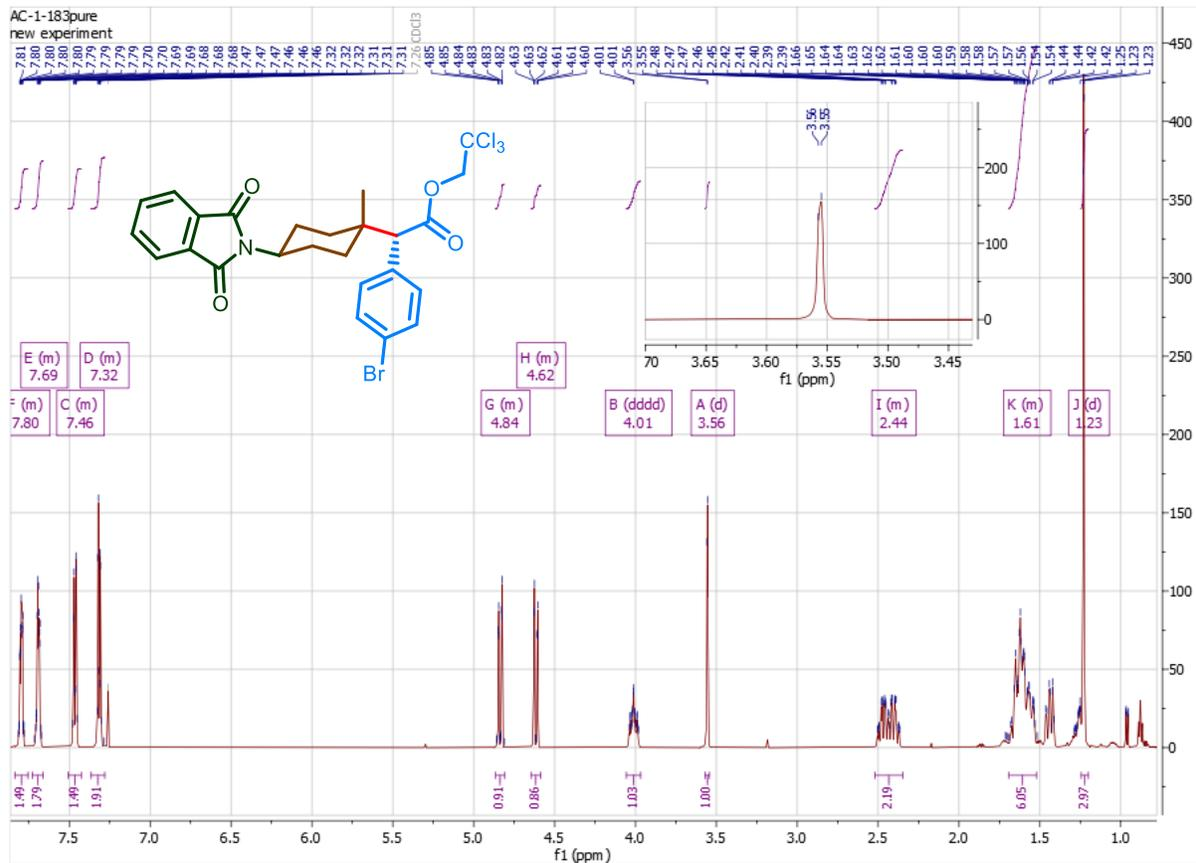
**Figure 2.15 Purified NMR for the Reaction with a mixture of *cis* and *trans* isomers (50:50) of 4-methylcyclohexylamine Derivative**
