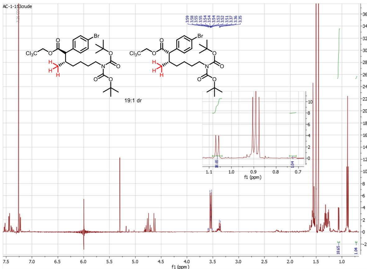
**Figure 2.5 Crude NMR for the Reaction with bis N-Boc Protected Substrate**
