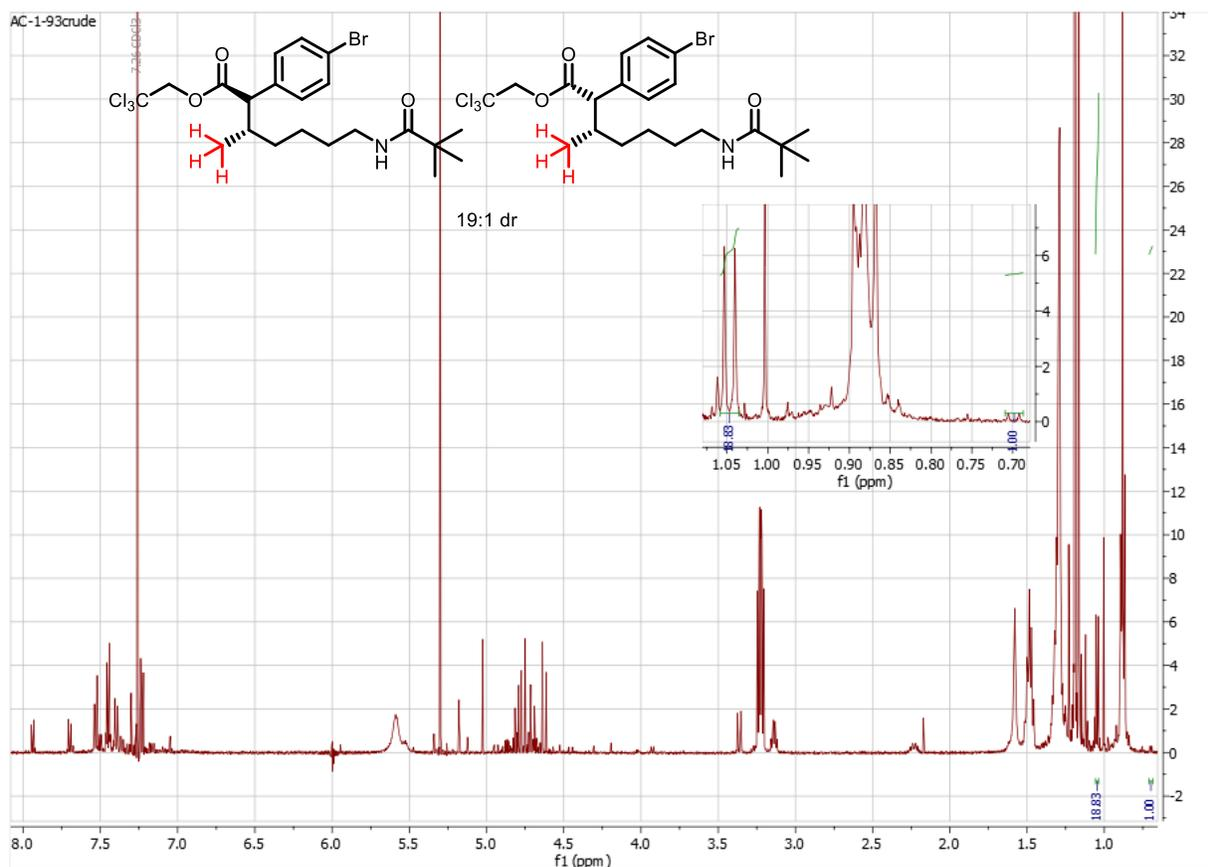
**Figure 2.3 Crude NMR for the Reaction with Trimethylacetamide-Protected Substrate**
