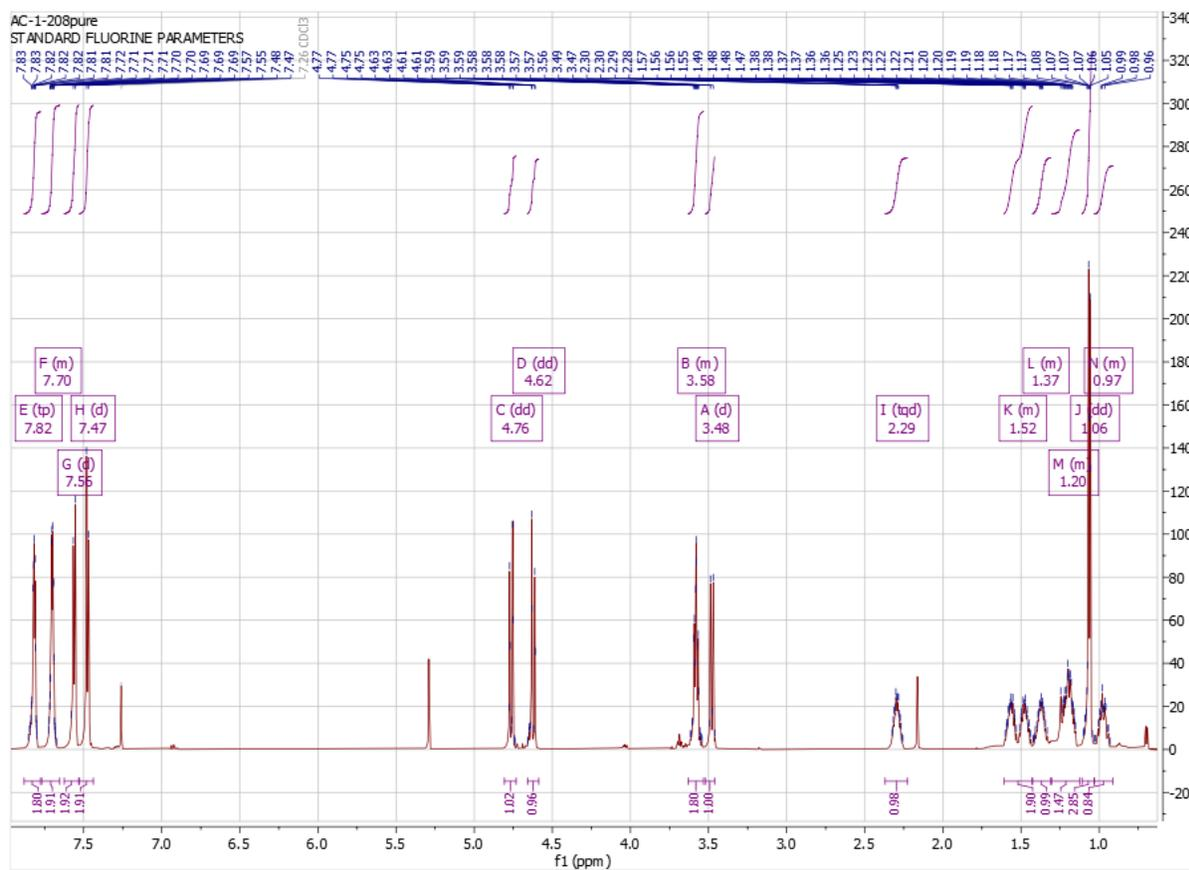
Figure 2.24 Purified NMR for *p*-CF<sub>3</sub> phenyldiazoacetate
