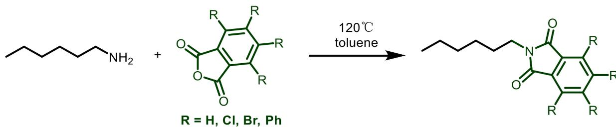
To a 50 ml of clean round-bottom flask equipped with a large egg-shaped magnetic stir-bar, phthalic anhydride/its derivatives (0.01 mol, 1.0 equiv.) and hexylamine/hydrocarbons with primary amine (0.01 mol, 1.0 equiv.) were added. Then, to the RBF with two substrates, dimethylformamide (20 ml) is added. The contents are stirred and heated to 120°C under a
