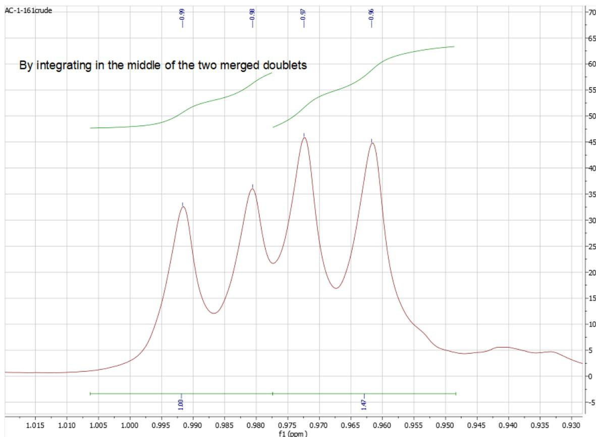
**Figure 2.19 Integrating by Cutting in the Middle of the Merged Doublets**
