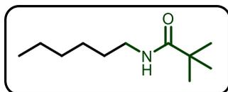
Dissolve 10mmol (1.0 equiv) of hexylamine in acetonitrile and cool the mixture to  $0^\circ\text{C}$  in an ice water bath. Add triethyl amine (20mmol, 2.0 equiv) and pivalic anhydride (40mmol, 4.0 equiv)
