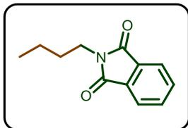
The product was obtained by general procedure (1). The silica gel chromatography was run by Biotage with 20% EtOAc/Hexane.  $^1\text{H}$  NMR (600 MHz,  $\text{cdCl}_3$ )  $\delta$  7.87 – 7.78 (m, 2H), 7.73 – 7.67 (m, 2H), 3.68 (t,  $J = 7.4$  Hz, 2H), 1.69 – 1.60 (m, 2H), 1.41 – 1.31 (m, 2H), 0.94 (t,  $J = 7.4$ , Hz, 3H).
