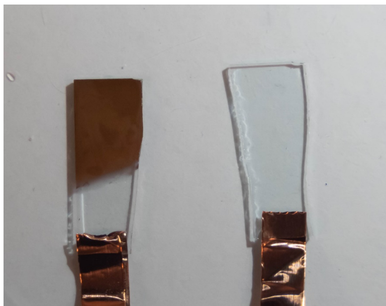
Figure 3.9. Electrodeposited Au on ITO disc electrode Before deposition(right), after deposition (left)
