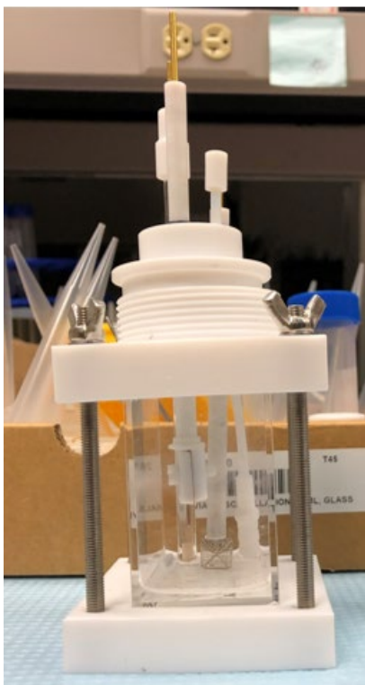
Figure 3.6. Raman spectro-electrochemical cell-02
