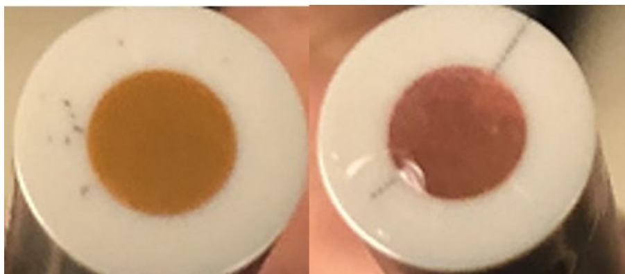
Figure 3.10. Electrodeposited Cu on Au disc electrode Before deposition(left), after deposition (right)
