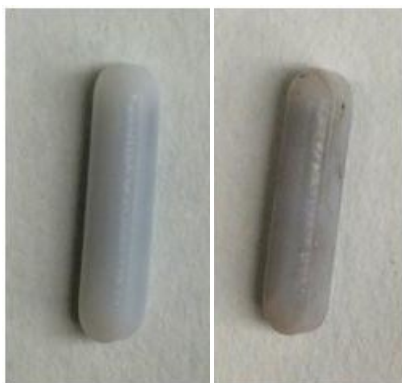
Figure 8-12 Photographs of the magnetic stir bar before (left) and after (right) photocatalytic hydrogen evolution for 5 hrs. Conditions: LED light (20 mW, 455 nm, beam diameter ~0.4 cm), [Ir(ppy) 2 (dtbbpy)] + (0.2 mM), TEOA (0.25 M), H 2 O (1.4 M), catalyst (320 μM NiCl 2 ), 2 mL CH 3 CN/DMF (1/3) deaerated with Ar.
