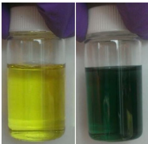
Figure 7-6 Photographs of the photocatalytic reaction solution before (left) and after (right) illumination. Conditions: LED light (20 mW, 455 nm, beam diameter ~0.4 cm), [Ir(ppy) 2 (dtbbpy)] + (0.2 mM), TEOA (0.25 M), catalyst Ni 4 P 2 (20 μM) in 2 mL CH 3 CN/DMF (1/3) deaerated with Ar.
