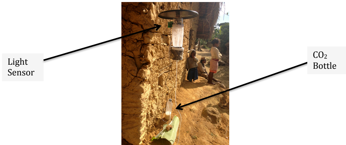
Figure 2. Example of CDC miniature light trap setup, in six villages near Ranomafana National Park, Madagascar
