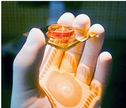
**Figure 2.1: Substrate-integrated microelectrode arrays.** Micro-electrode array (MEA) is embedded in a glass dish. Shadows on hand reveal leads radiating from micro-electrodes. In addition to providing multichannel electrophysiological measurements, this system provides excellent pharmacological, genetic, and optical accessibility. Image source: [Potter, 1998](#).
