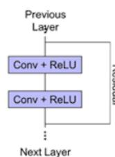
Figure 3. (A) Schematic diagrams of the baseline CNN, Inception V3, and ResNet. The Inception (B) and Residual (C) are used as building blocks for the Inception and ResNet architectures, respectively. Adapted from Christopher et al., 2018.
