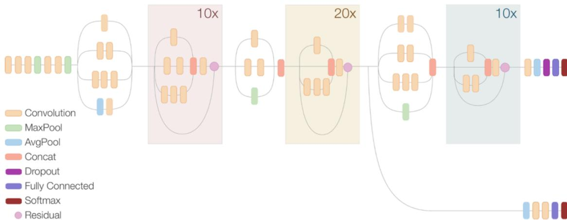
Figure 4. Schematic diagram of Inception-ResNet V2. Adapted from
