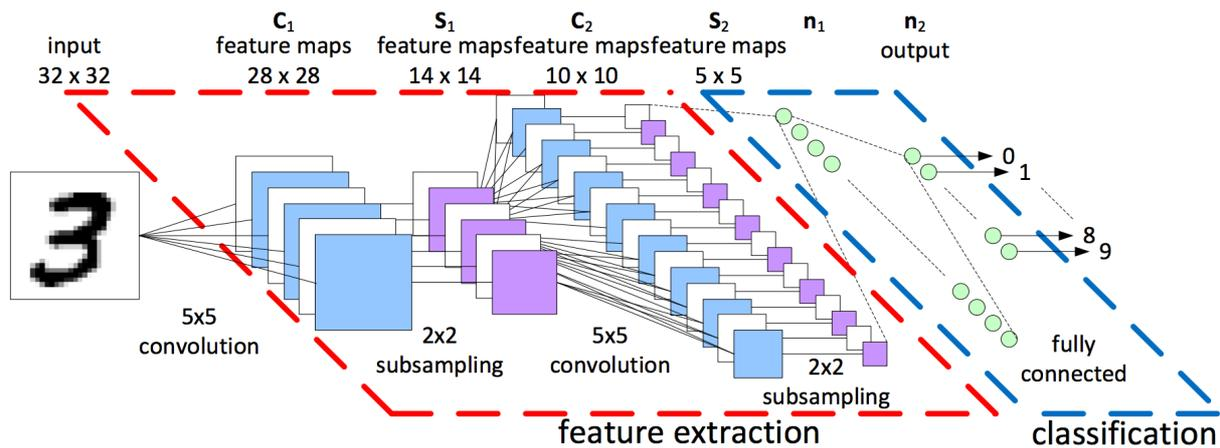
Figure 1. Typical structure of CNN model with 2 convolutional layers and 2 pooling (subsampling) layers followed by fully connected layers. Adapted from <https://github.com/tavgreen/cnn-and-dnn>.
