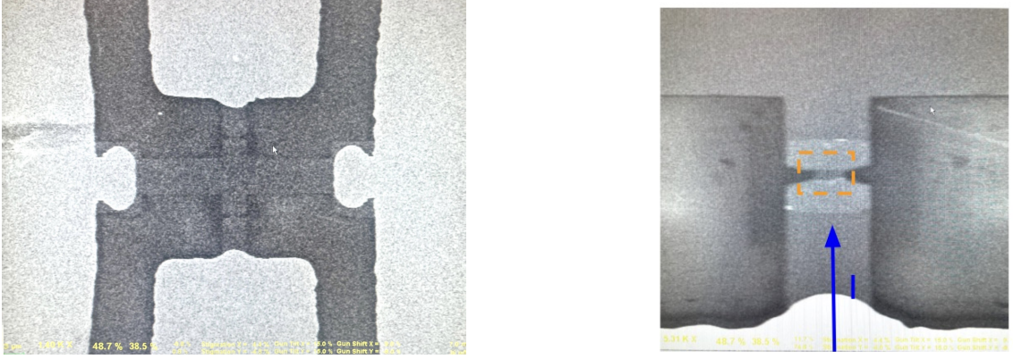
Figure 2.2: Left: SEM image of the leads and the \beta -Ta strip; Right: magnified SEM image of the flare-out design for precise \beta -Ta strip geometry. The length of the \beta -Ta strip is 500 nm, width is 1500 nm, and thickness is 10 nm. (Orange rectangle: circles out \beta -Ta strip; blue line: the direction that current flows)
