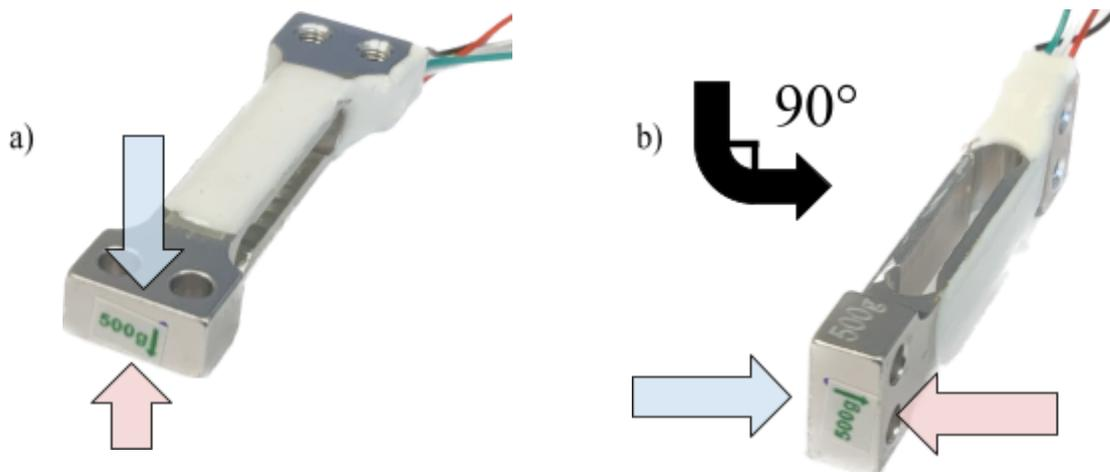
Figure 2.6: Pushing down (blue arrow) on the load cell on the left (a), gives us a downward force, while pushing upward (red arrow) gives an upward force. Another load cell load cell turned 90 degrees (b) measures right (blue arrow) and left (red arrow) force.
