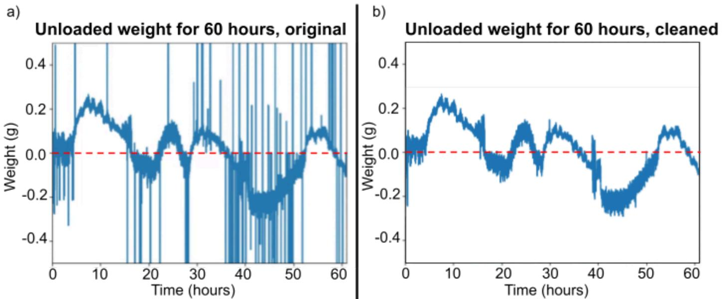
Figure 2.7: Noise measurements for an unloaded weight for 60 hours of noisy original data (a) and cleaned data (b). The red dotted line indicates where weight = 0g.
