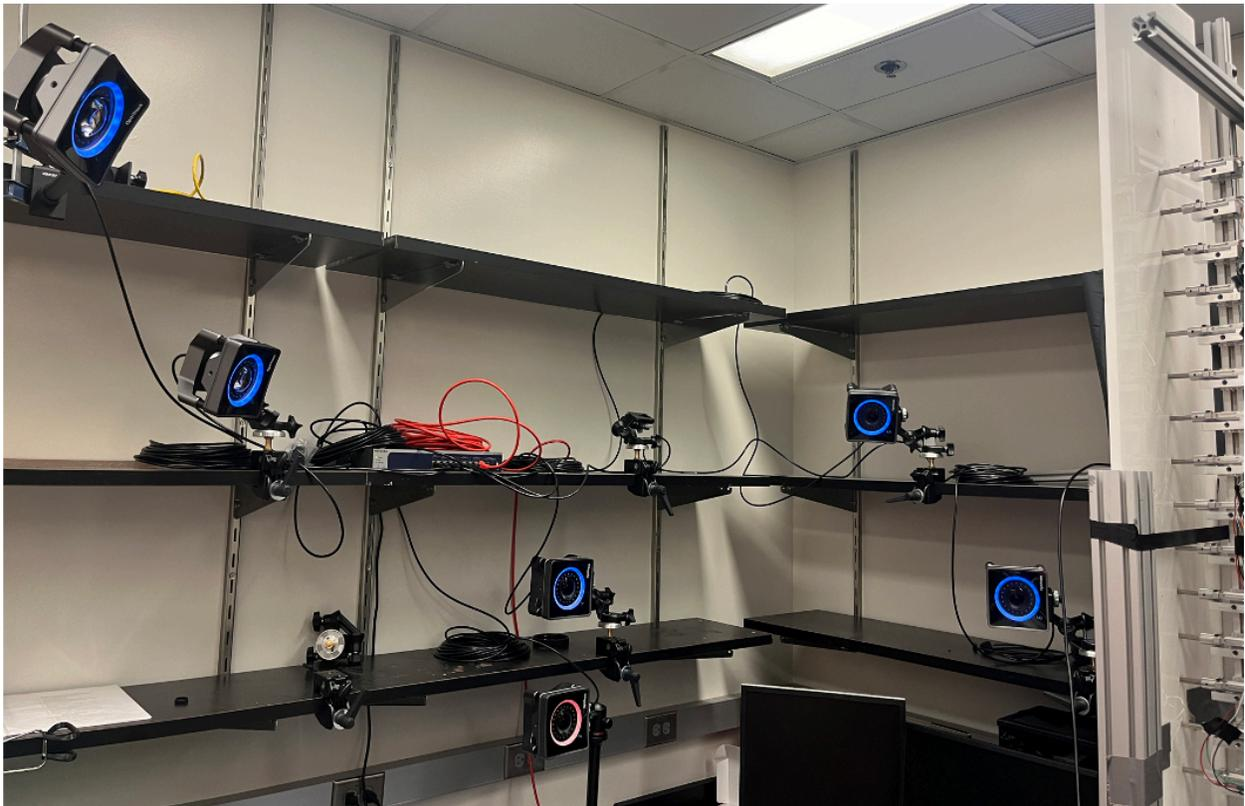
Figure 2.9: Optitrack camera setup facing the climbing wall.
