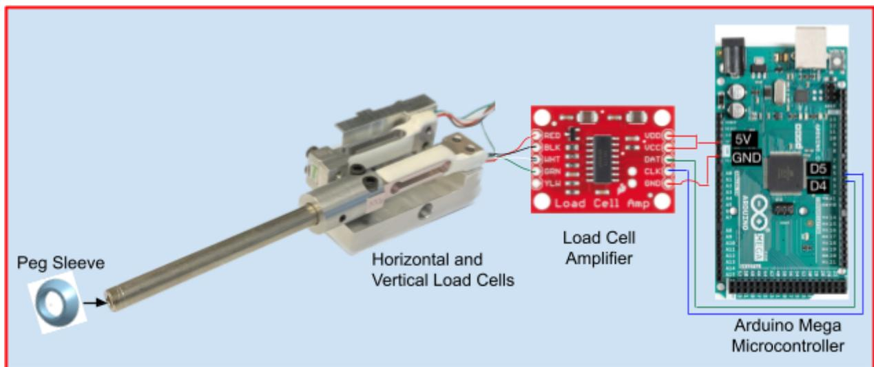
Figure 2.10: The entire experimental setup
