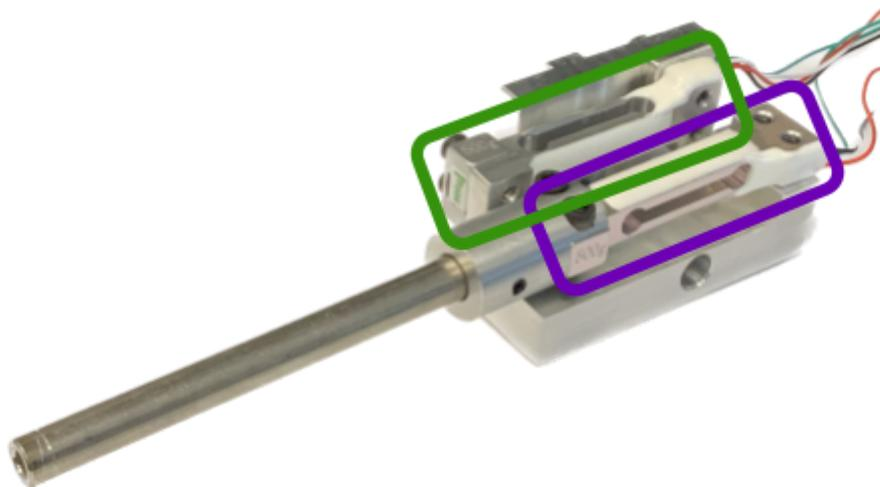
Figure 2.4: Peg setup with 2 load cells. The load cells are held together by custom metal housing. The green box indicates the load cell that measures vertical forces, while the purple box indicates the one that measures horizontal forces.
