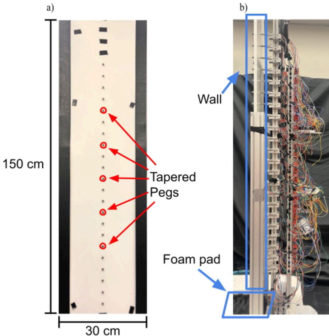
Figure 2.1: Front (a) and side view (b) of 150 x 30 cm vertical climbing wall setup with 22 force sensing pegs, with tapered pegs circled in red, and the foam pad and wall boxed in blue.
