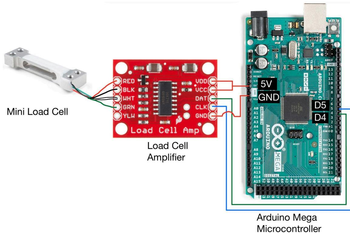
Figure 2.3: Example miniature load cell setup: A mini load cell [\[11\]](#) is connected to an amplifier [\[12\]](#), which is connected to an Arduino Mega microcontroller [\[13\]](#).
