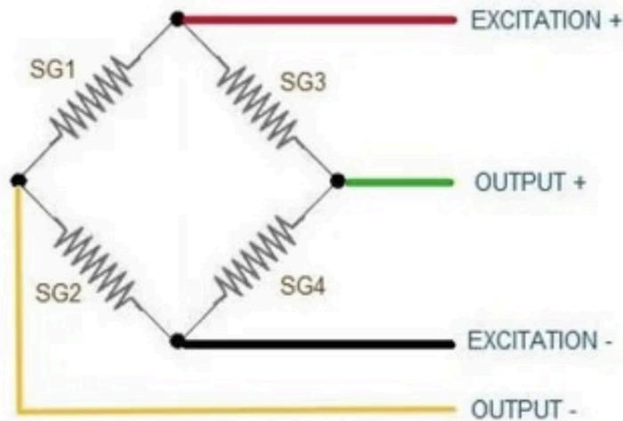
Figure 2.5: Bridge circuit of four resistors in each of the load cells [\[14\]](#).
