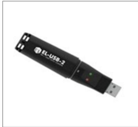
Figure 2. Device used to measure the temperature and humidity of homes ( EL-USB-2 Lacar Humidity and Temperature USB )
