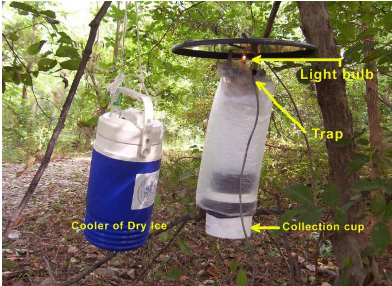
Figure 6. Diagram of a light trap courtesy of Fairfax County Health Department.
