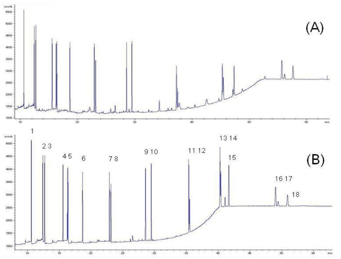
Figure 2-6 GC-FID chromatogram of the 18 PAHs. X-axis = time (min). Y-axis = area counts. 1, naphthalene; 2, 1-methylnaphthalene; 3, 2-methylnaphthalene; 4, acenaphthylene; 5, acenaphthene; 6, fluorene; 7, phenanthrene; 8, anthracene; 9, fluoranthene; 10, pyrene; 11, benz(a)anthracene; 12, chrysene; 13,
