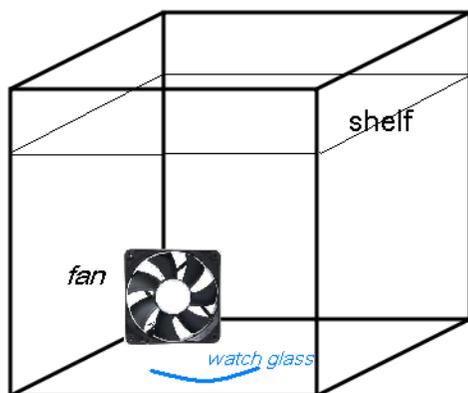
Figure 2-4 Schematic diagram of the static chamber
