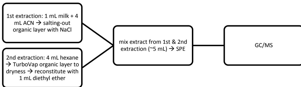
Figure 3-7 Flow diagram of the liquid-liquid extraction procedure followed by SPE and GC analysis
