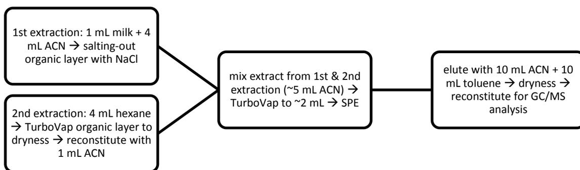
Figure 3-10 Flow diagram of the modified liquid-liquid extraction and SPE procedure
