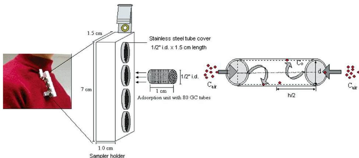
Figure 2-2 Schematic diagram of the passive sampler and its diffusion process (Fan et al. 2006)<sup>33</sup>
