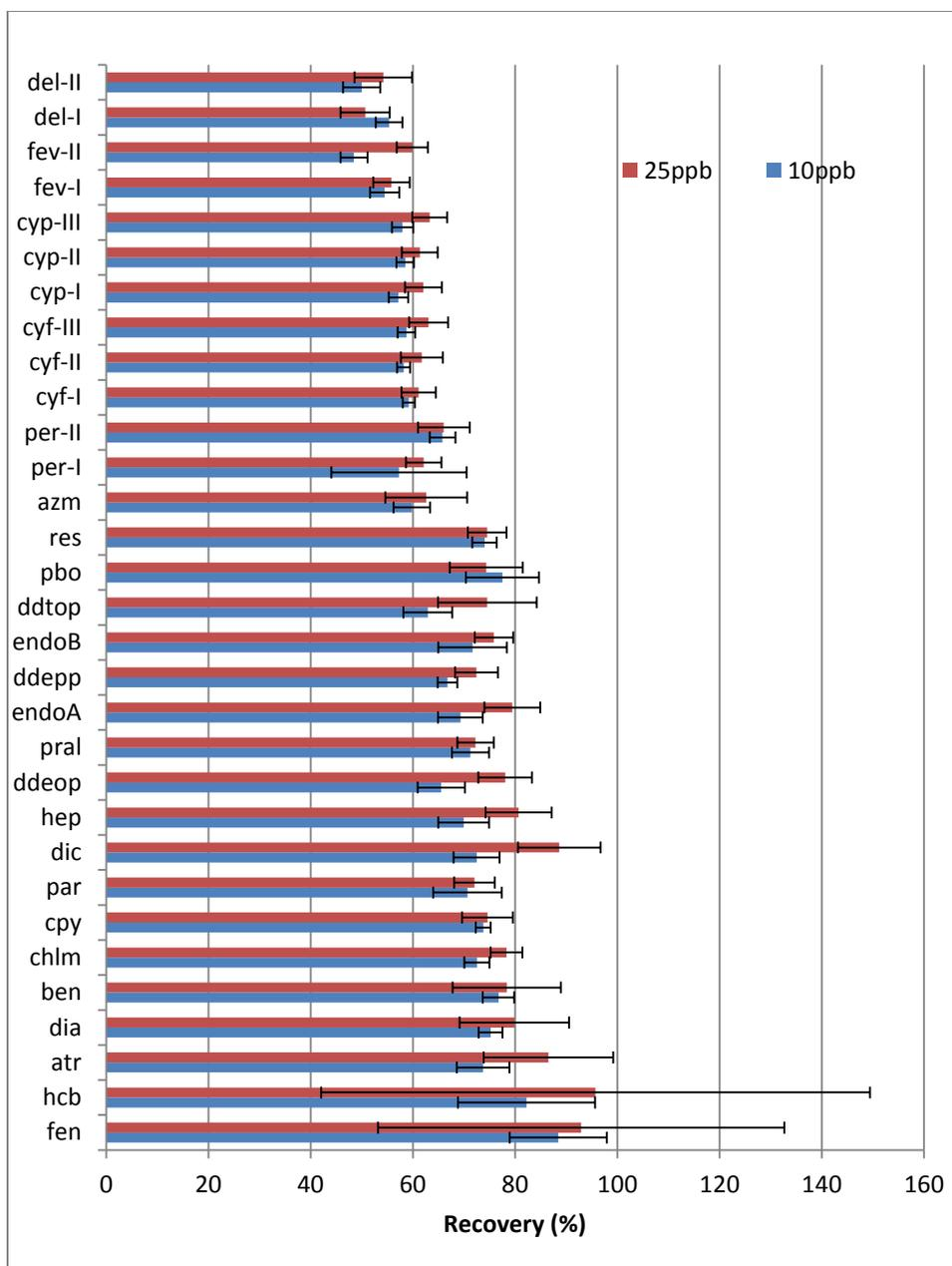
Figure 4-1 Recoveries of described method at 25 ppb and 10 ppb
