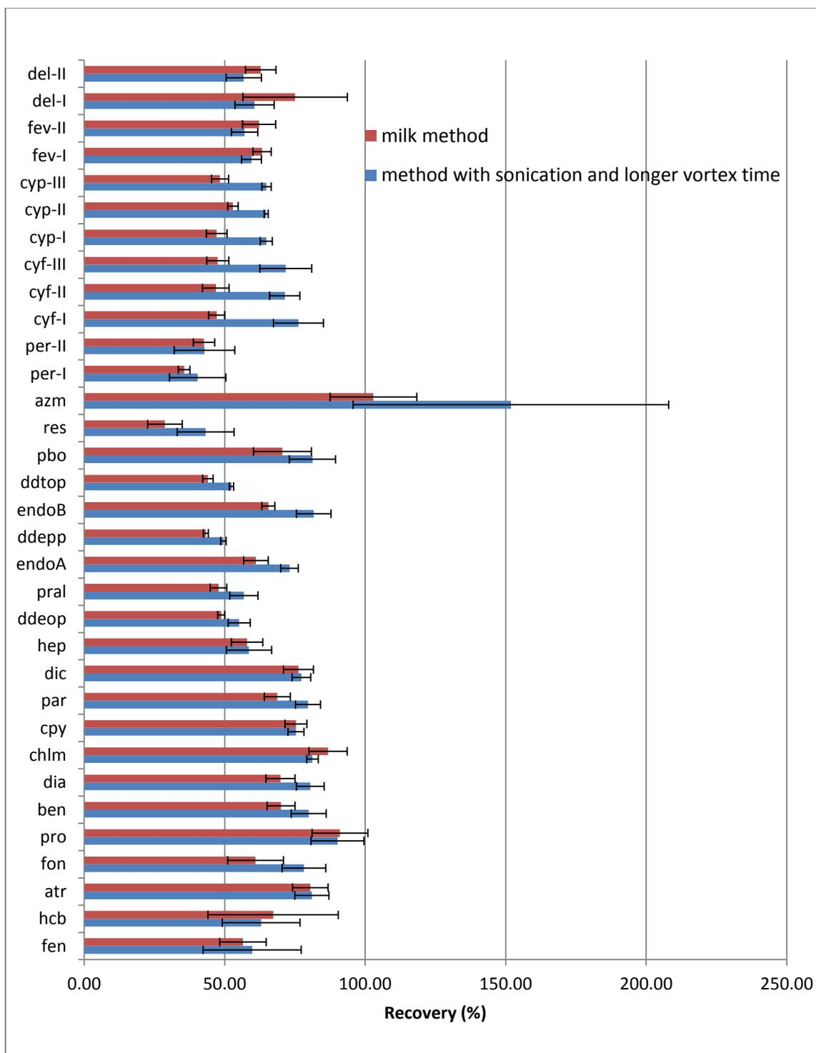
Figure 3-16 recoveries of two different methods for baby formulas at the concentration level of 25 ppb
