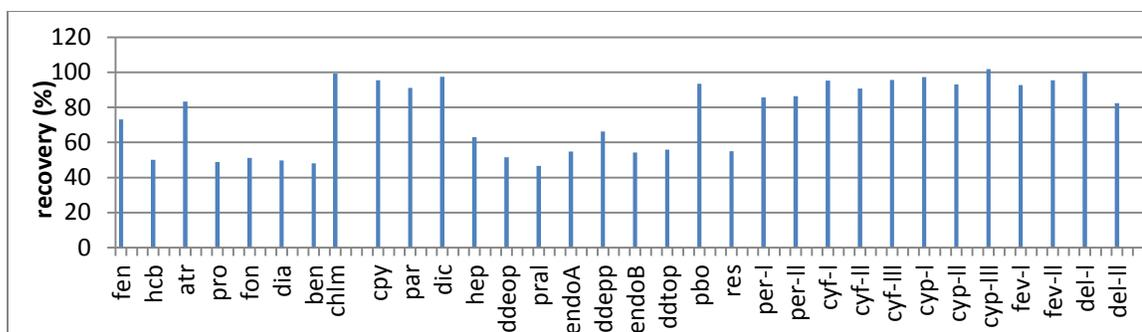
Figure 3-8 Recoveries (%) with the Dual-Layer Envi-Carb II/PSA 500/300mg 6mL SPE tubes.
