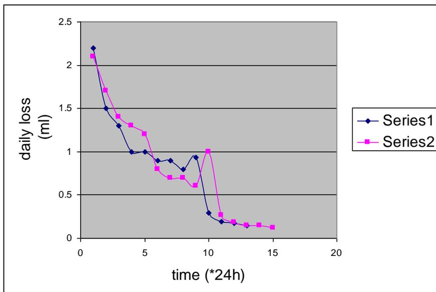
Figure 2-5 Daily loss of ethyl acetate to check the leakage rate of the static chamber
