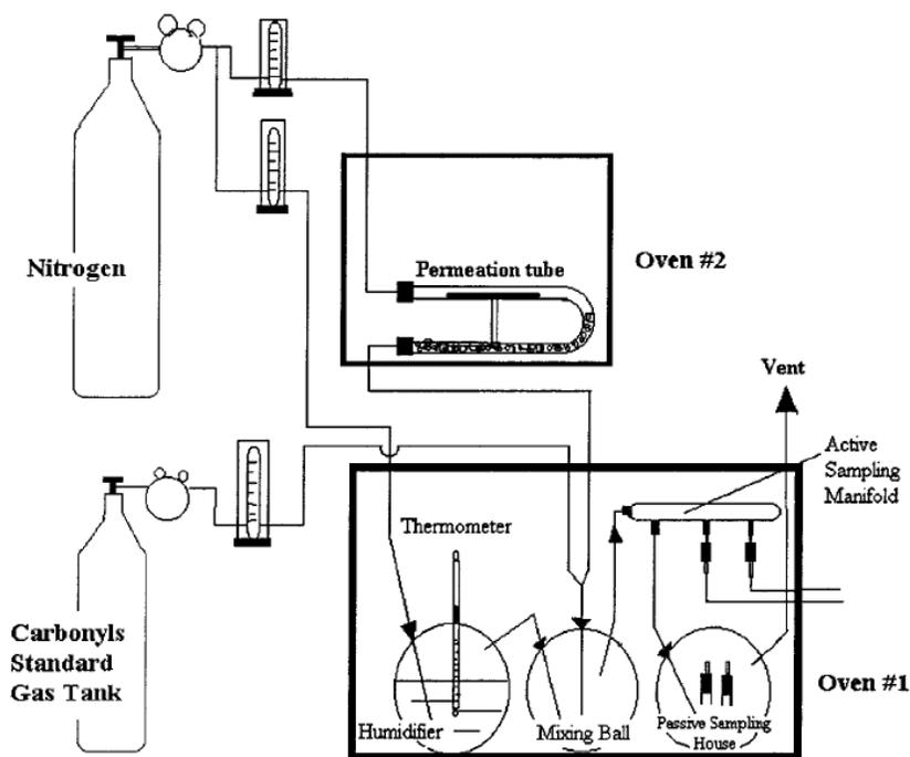
Figure 2-3 Dynamic dilution system for generation of a controlled test atmosphere
