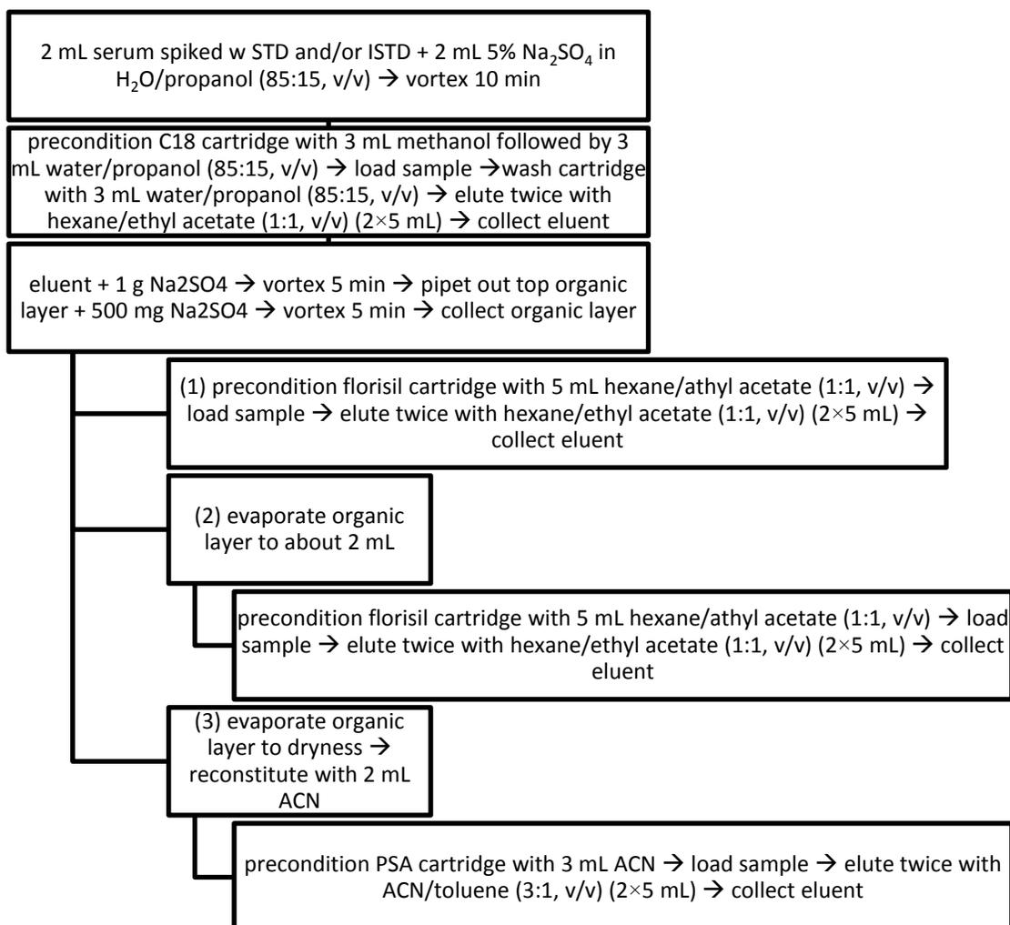
**Figure 4-3 Flow diagram of three extraction methods that were modified from the one in Conka et al.<sup>119</sup>**
