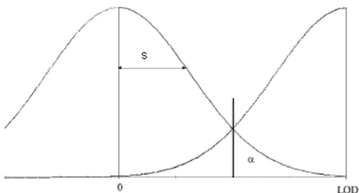
Figure 3-17 Graphical representation of the limit of detection<sup>99</sup>
