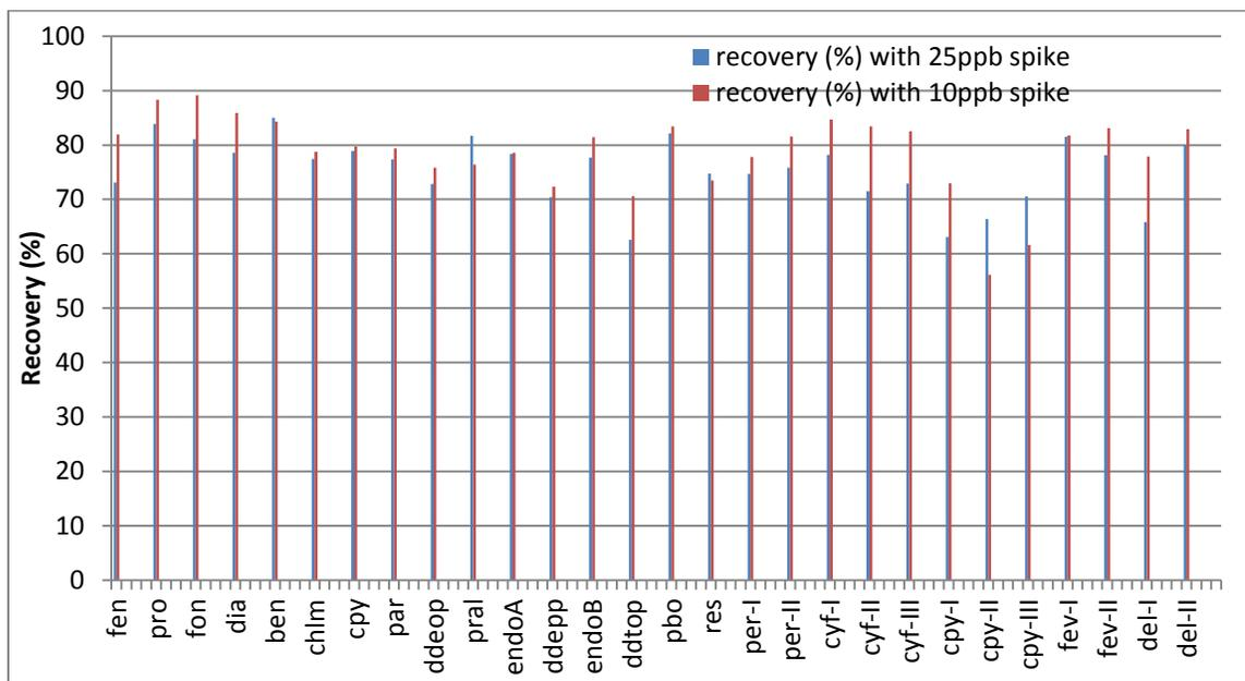
Figure 3-13 Recoveries at two different spiking levels
