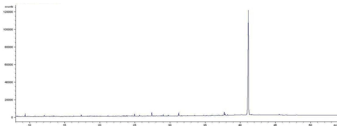
Figure 2-13 GC-FID chromatogram of the 18 PAHs with the unidentified peak. X-axis = time (min). Y-axis = area counts.
