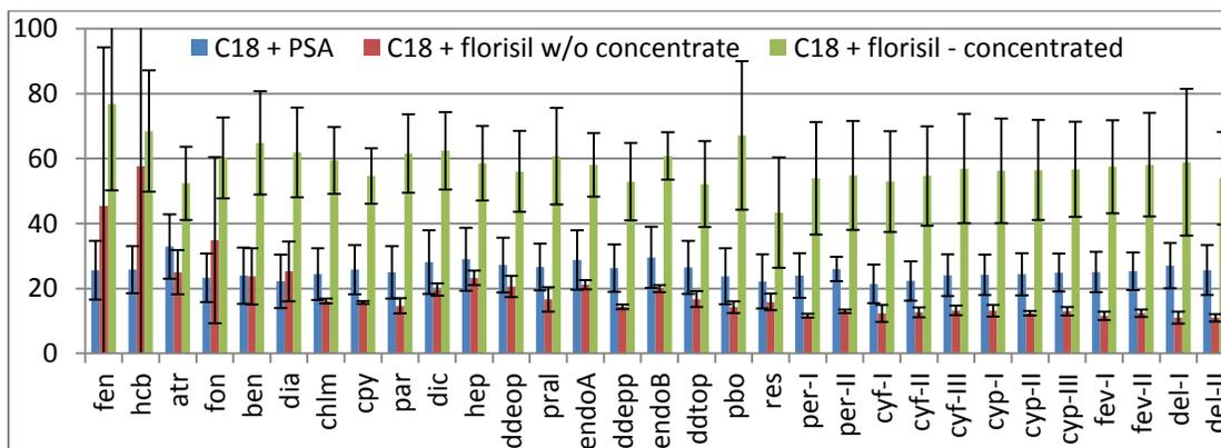
Figure 4-5 Recoveries of three extraction methods. Blue, red, and green bars represent extraction methods (3), (1), and (2) described in Figure 4-3. Y-axis represents the percent recovery (%).
