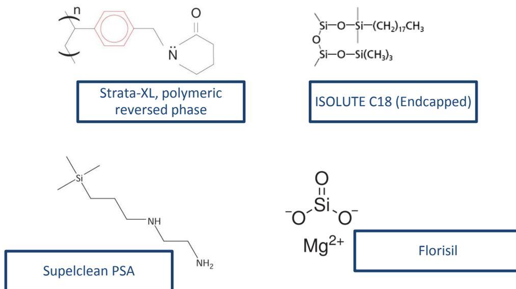
Figure 4-4 Chemical structures of four representative SPE packing in this study
