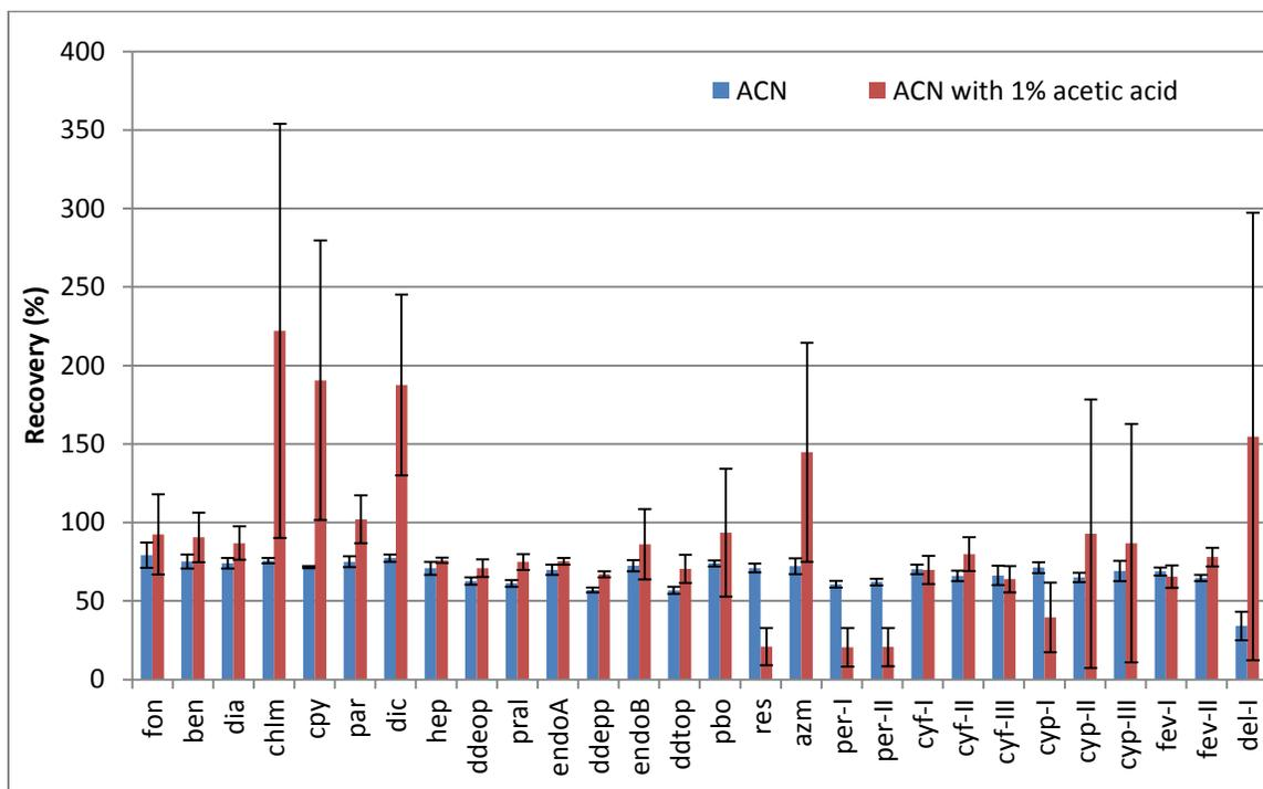
Figure 3-14 Recoveries of two sample preparation methods. Blue and red bars represent the first extraction with acetonitrile and 1% acetic acid acetonitrile respectively.
