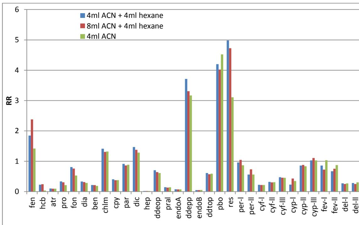
Figure 3-6 Comparison of RR among 3 different liquid-liquid extraction methods. Blue, red, and green bars represent method (1) extract with 4 mL ACN first and then 4 mL hexane, method (2) extract with 8 mL ACN first and then 4 mL hexane, and method (3) extract with 4 mL ACN only, respectively.
