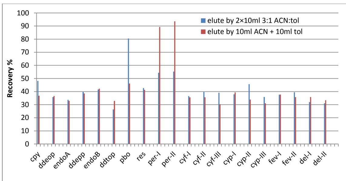
Figure 3-12 Recoveries of 500mg 6ml PSA cartridges without matrices
