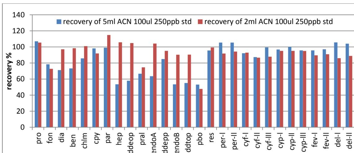
Figure 3-11 the comparison of recoveries from two different groups of samples. Blue and red bars represent group 2 and 1 samples respectively.
