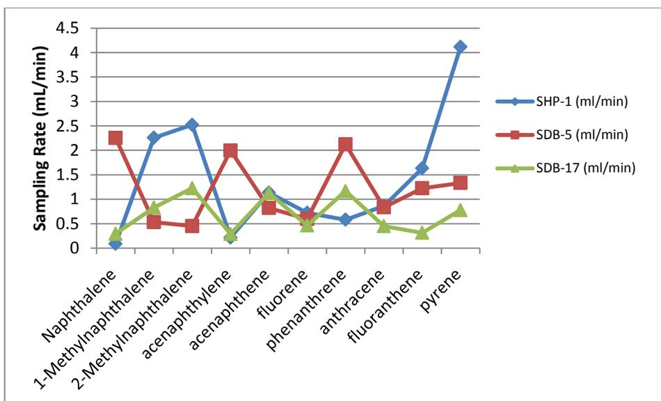
Figure 2-8 Sampling rate of HP-1, DB-5 and DB-17 passive samplers in separate trial
