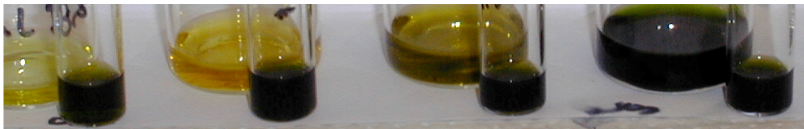
Figure 15. From left to right the ratio of \text{Cu}^{2+} to \text{Br}^- increases. The unexposed solutions are in the background while the solutions exposed to simulant CEES are in the smaller vials. The color change is maximized for the second vial from the right, in which the mol ratio of \text{Cu}^{2+} : \text{Br}^- is 1 : 2.
