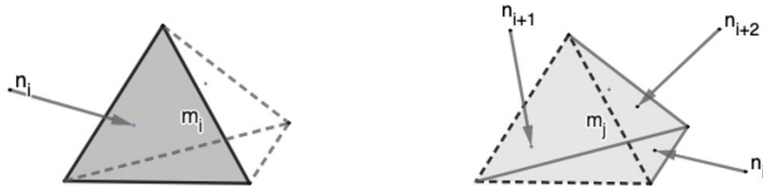
Figure 4.3: The left side shows a tetrahedral element with domain m_i and one surface boundary n_i (displayed by the solid lines and shaded region). On the other hand, with proper modifications, the same element is now reassigned to domain m_j and contains three different surface boundaries n_i, n_{i+1}, n_{i+2} . Notice that the label n_i is different in both instances.[4]
