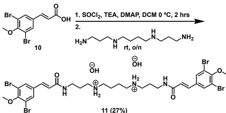
**Scheme 15.** Synthesis of protonated ianthelliformisamine C (**11**) through the formation of the acyl chloride derivative of **10**.
