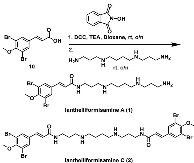
**Scheme 8.** DCC coupling with hydroxyphthalimide, **10**, and spermine to synthesize **1** and **2**.
