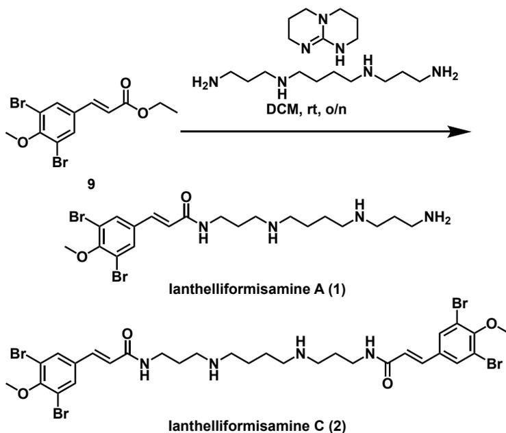
**Scheme 14.** Amidation between **9** and spermine catalyzed by TBD to produce **1** and **2**.
