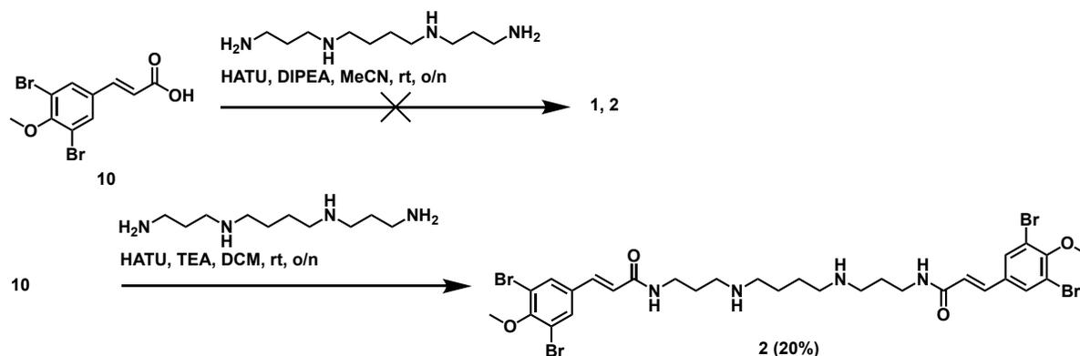
**Scheme 10.** Synthesis of **2** through an amide coupling with HATU.
