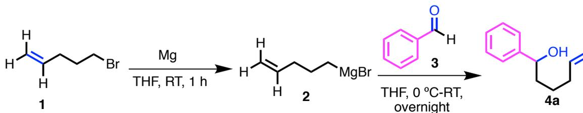
**Scheme 1.** Synthesis of acyclic monosubstituted alkenol **4a**.
