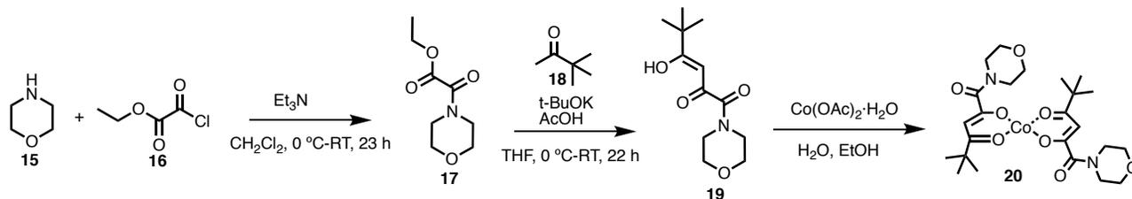
**Scheme 5.** Synthesis of  $\text{Co}(\text{MODP})_2$  catalyst.
